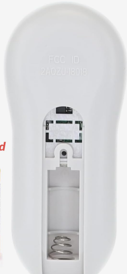
Figure 5: Battery installation. This diagram illustrates the correct orientation for inserting the 23A 12-volt battery into the remote control's battery compartment.
