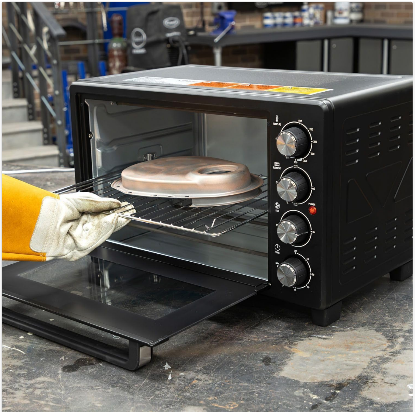
Figure 7: Curing a powder-coated part in the oven.
