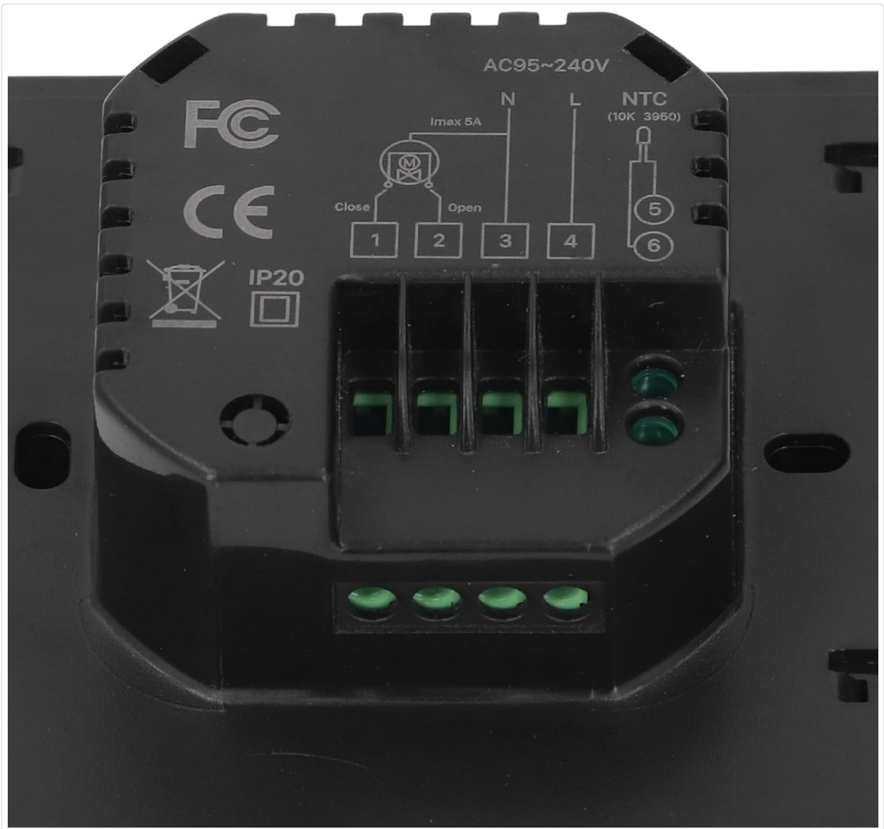
Image: Rear view of the thermostat illustrating the wiring terminals for power (N, L) and the NTC temperature sensor.
