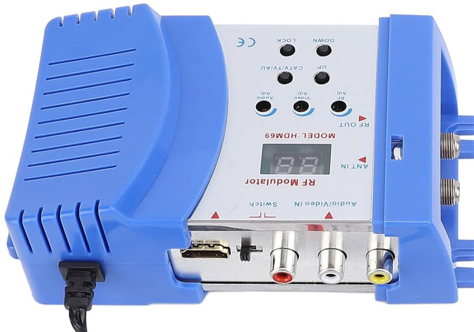
Image 4.1: Front view of the HDM69 Modulator, highlighting the input and control panel.
