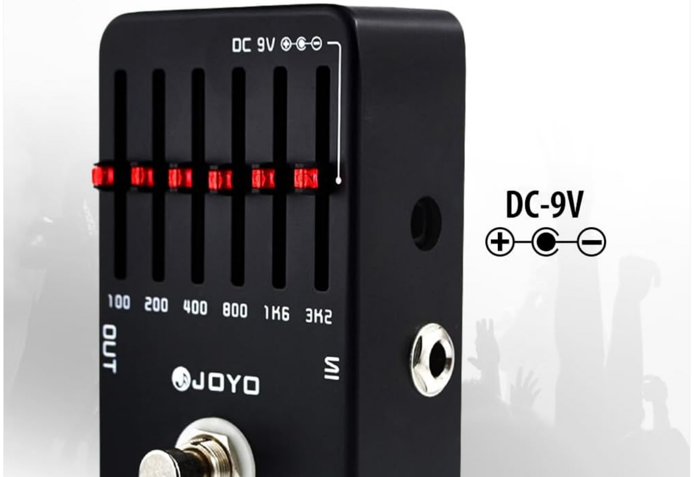
Image: Power Supply Note for the JOYO JF-11 EQ Pedal. This image visually explains the power connection, emphasizing the need for a DC 9V, center-negative adapter and recommending JOYO original or other reliable brands.
