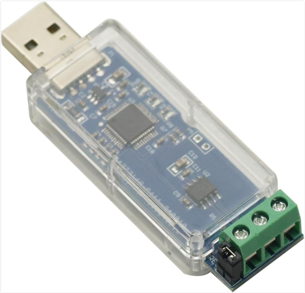
Figure 4.1: USB to CAN converter in operation with host software.
