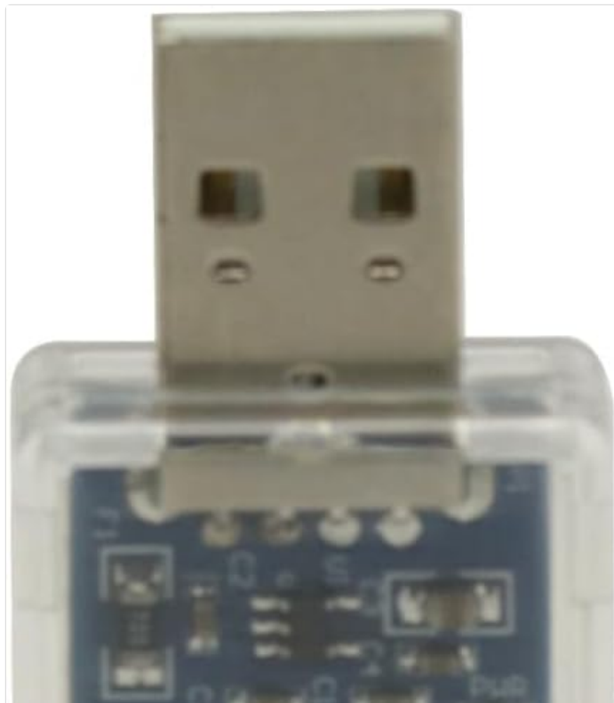
Figure 4.1: USB to CAN converter in operation with host software.
