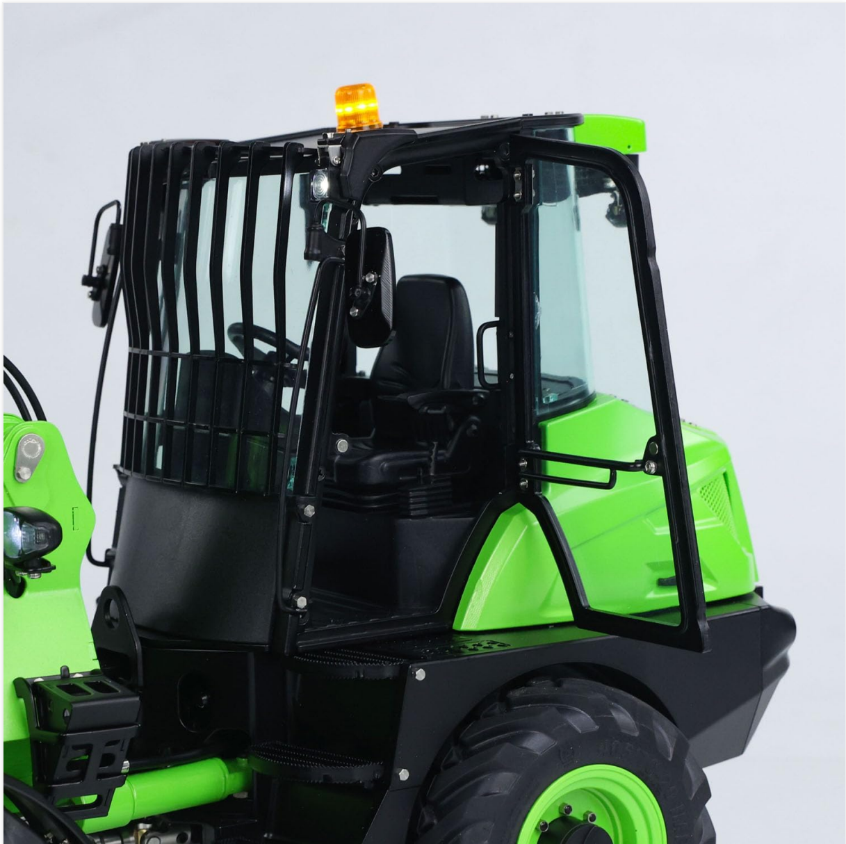
Figure 4.2: A detailed view of the loader's cab with the door open, showcasing the interior and the protective stainless steel cab guard.
