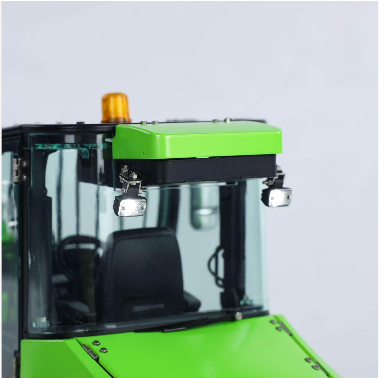
Figure 5.1: Detail of the loader's roof-mounted beacon light and front working lights, highlighting the integrated lighting system.
