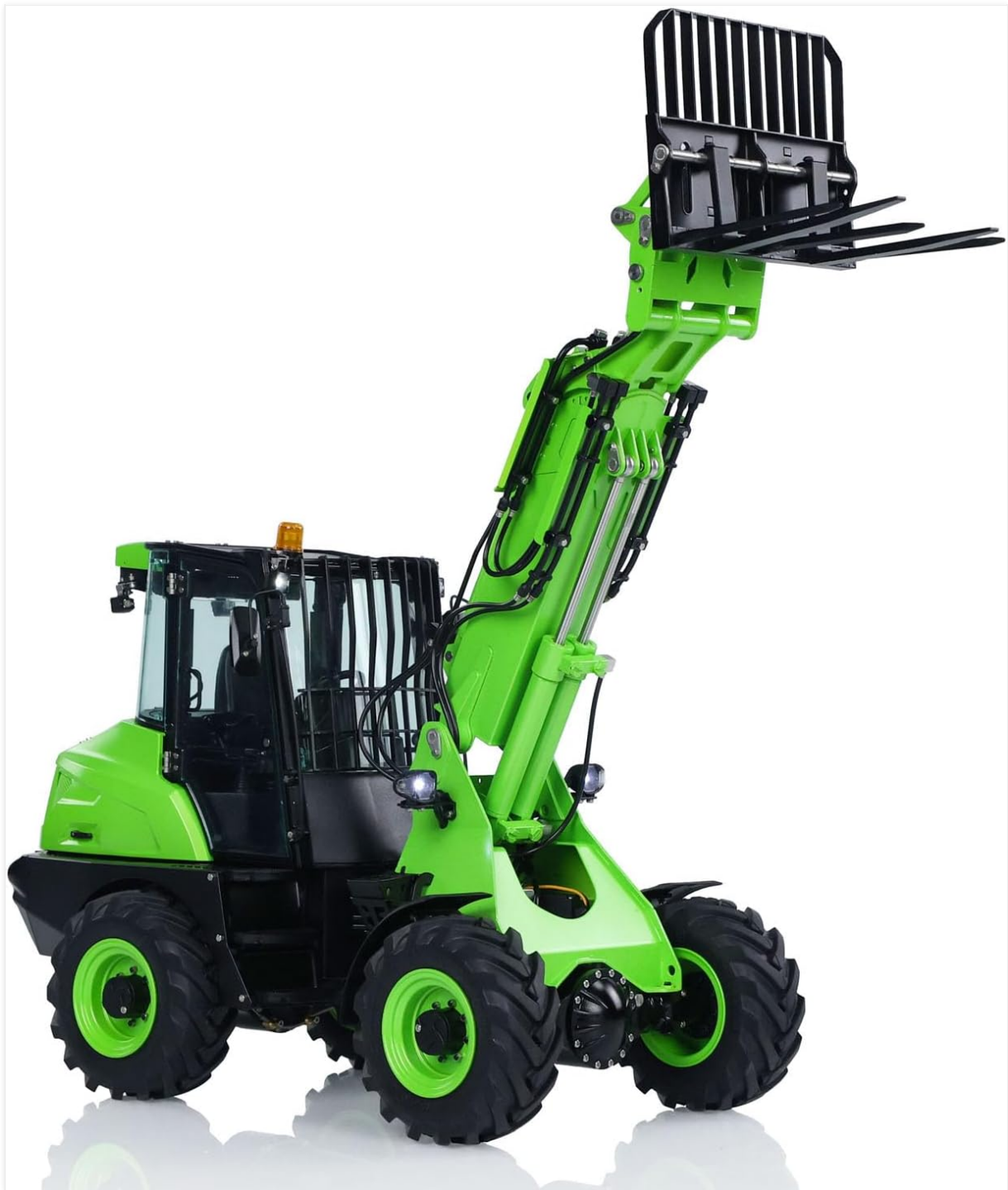
Figure 4.1: The LESU AT1050 with its telescopic arm fully extended and the fork attachment raised, demonstrating its reach and lifting capabilities.
