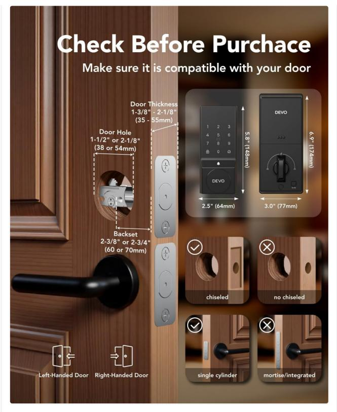
This diagram provides essential measurements and door type compatibility checks for installing the Devo G4 Smart Lock, detailing requirements for door thickness, bore hole diameter, backset, and confirming suitability for chiselled and single-cylinder doors.
