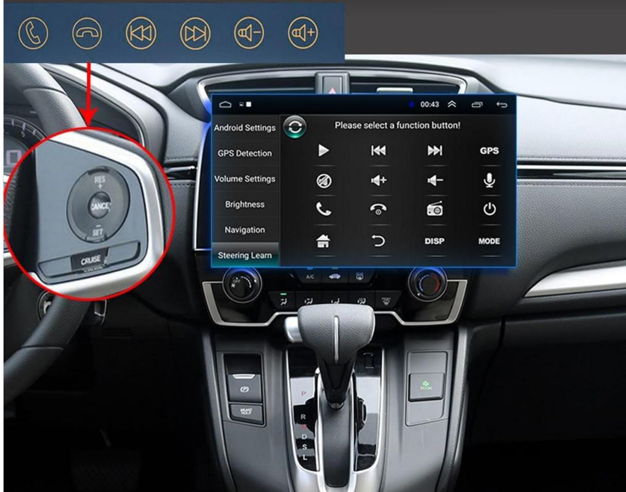
Image: Illustrates the process of setting up steering wheel controls, showing the 'Steering Learn' menu on the car stereo screen.
