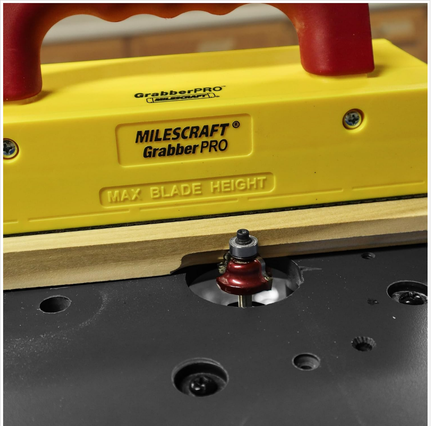
Image: The Milescraft GrabberPRO LITE guiding a wooden workpiece over a router bit on a router table.
