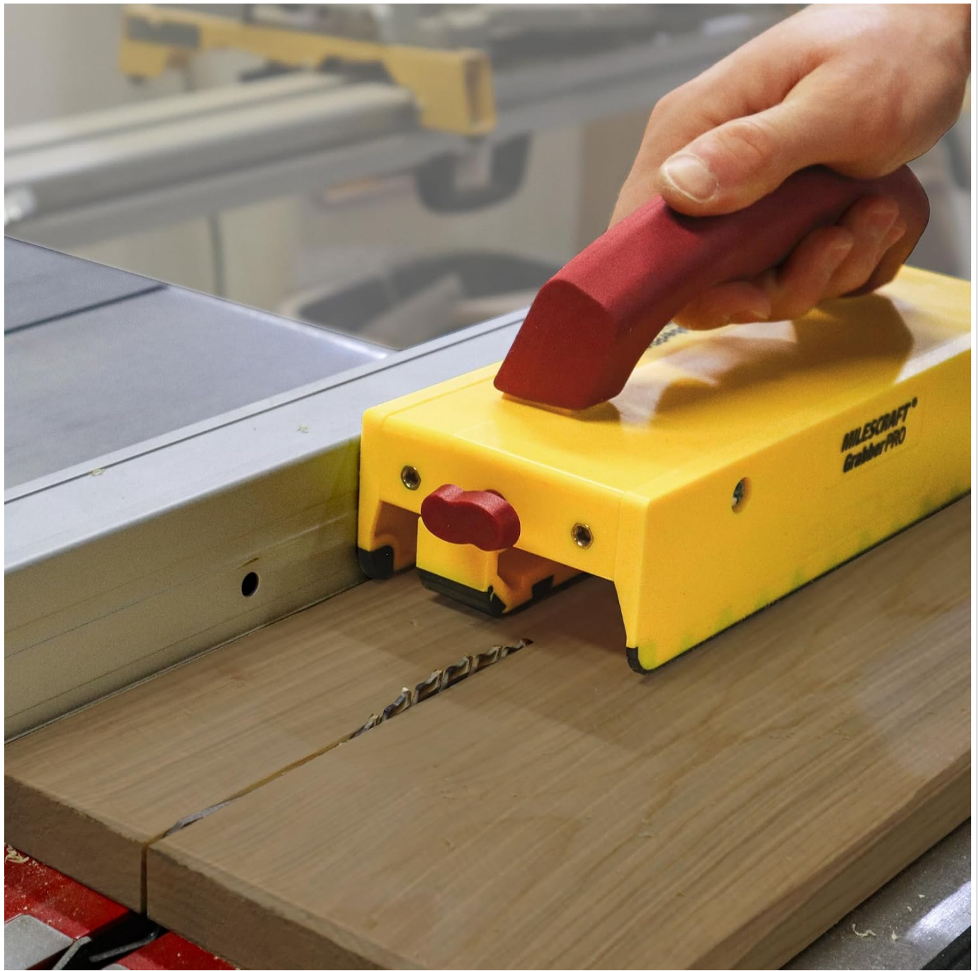
Image: A hand using the Milescraft GrabberPRO LITE to push a wooden workpiece through a table saw, demonstrating safe operation.
