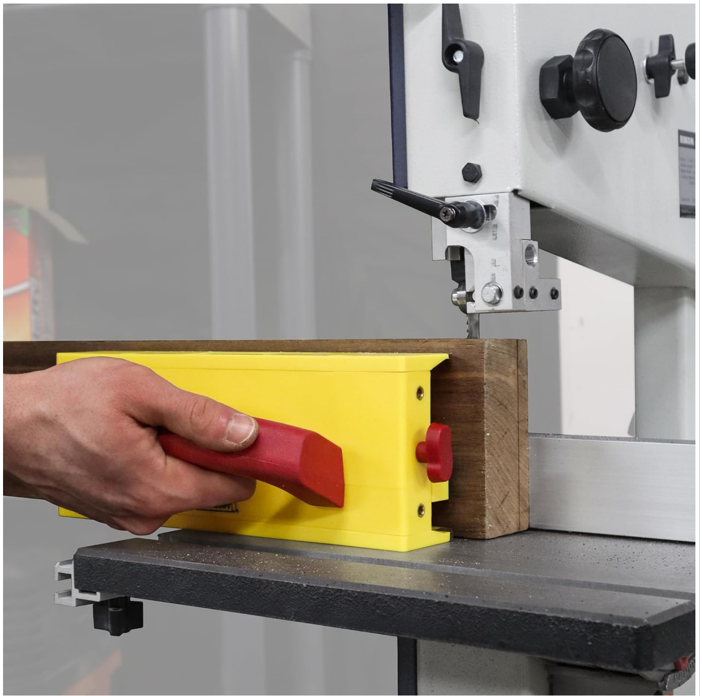
Image: A hand using the Milescraft GrabberPRO LITE to push a wooden board through a band saw, maintaining contact with the fence.
