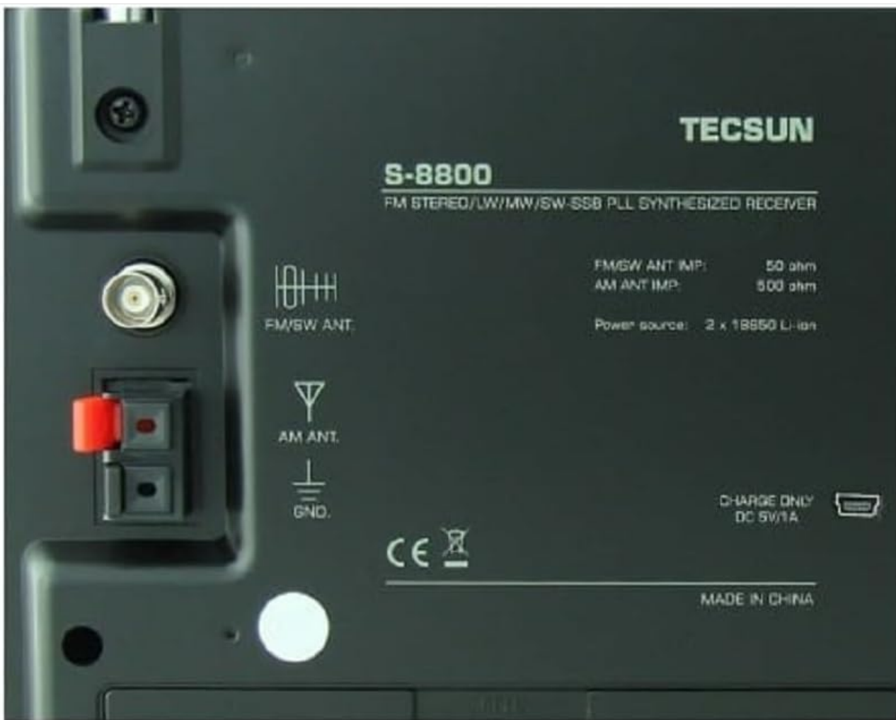
Figure 3.4: Rear panel with FM/SW BNC, AM/GND antenna terminals, and MiniUSB charging port.
