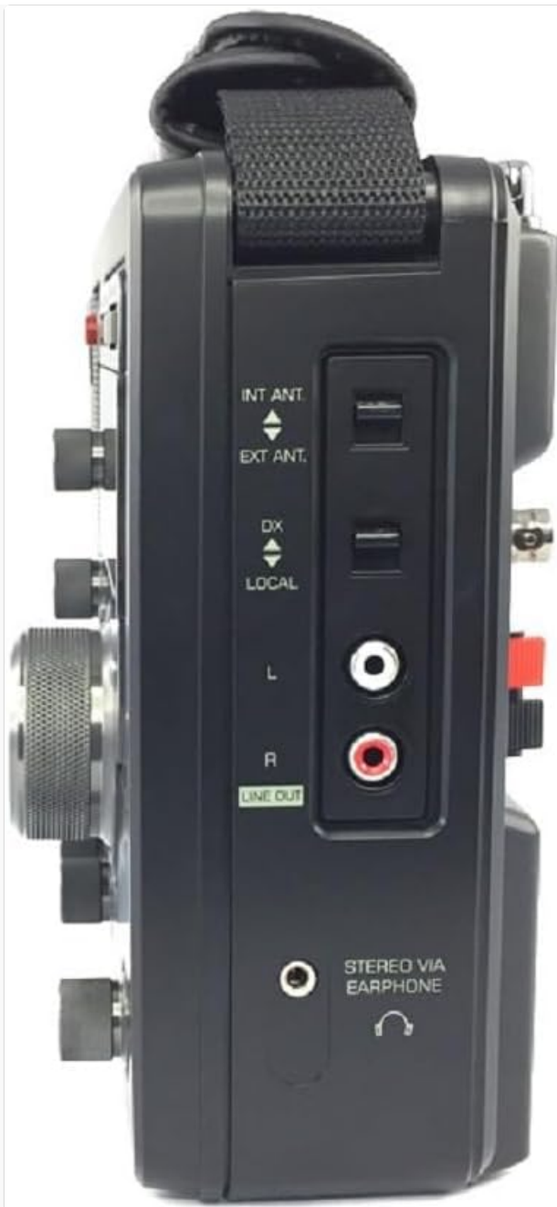
Figure 3.3: Side view illustrating headphone, line-out, and external antenna connections.
