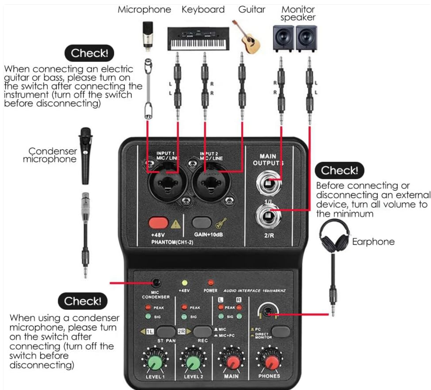
Figure 4: Connection diagram showing how to connect microphones, instruments (guitar, keyboard), monitor speakers, and headphones to the audio interface.
