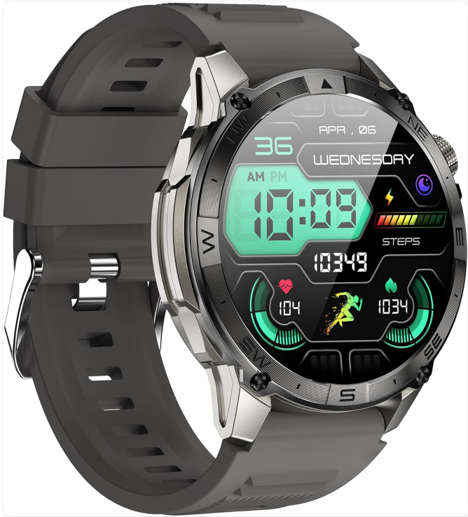
Figure 3.2: Front view of the VALDUS VG40 Pro Smartwatch, showcasing an alternative digital watch face. This display includes the current time, day, date, step count, heart rate, and battery status indicators.
