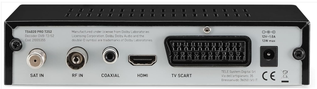
Figure 2: Rear panel connections of the TS4020 PRO decoder, including SAT IN, RF IN, Coaxial, HDMI, and TV SCART ports.
