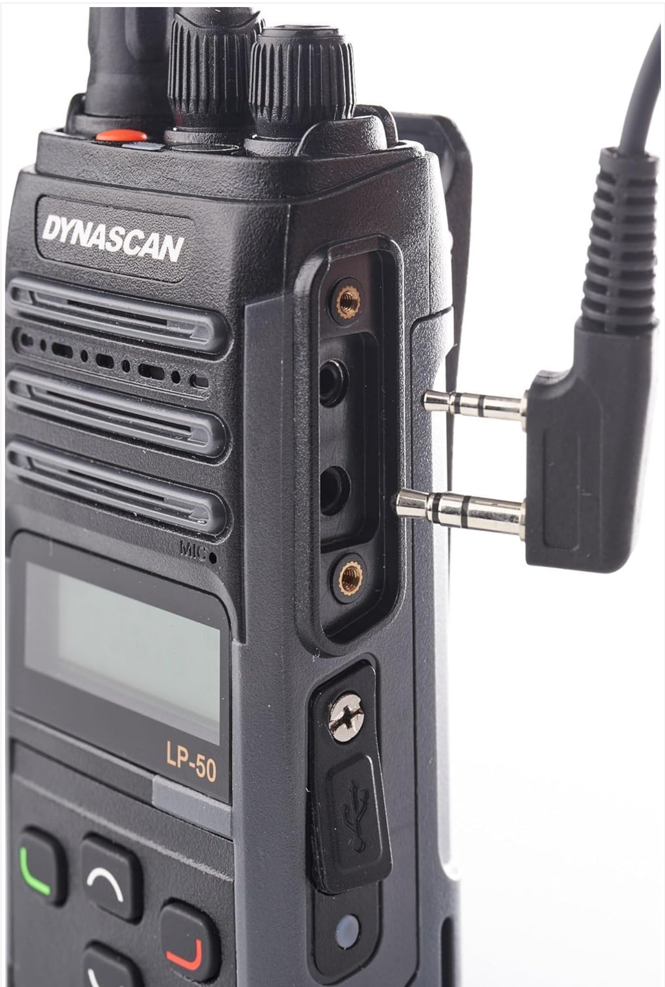
Figure 4.3: Side view of the LP-66, showing the dual audio accessory jacks for connecting external microphones or earpieces.
