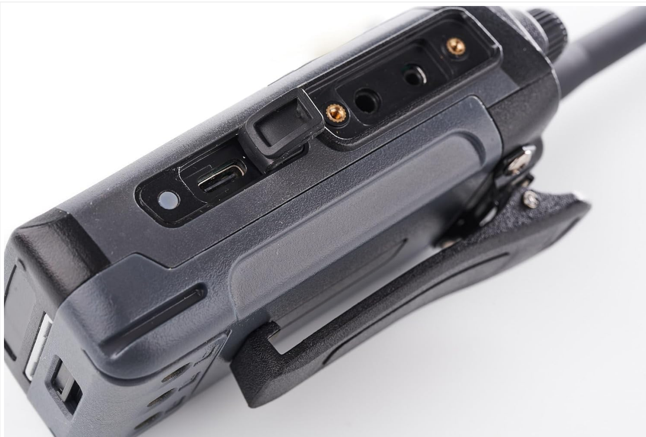
Figure 4.4: Another side view of the LP-66, illustrating the USB charging port and the attachment point for the belt clip.
