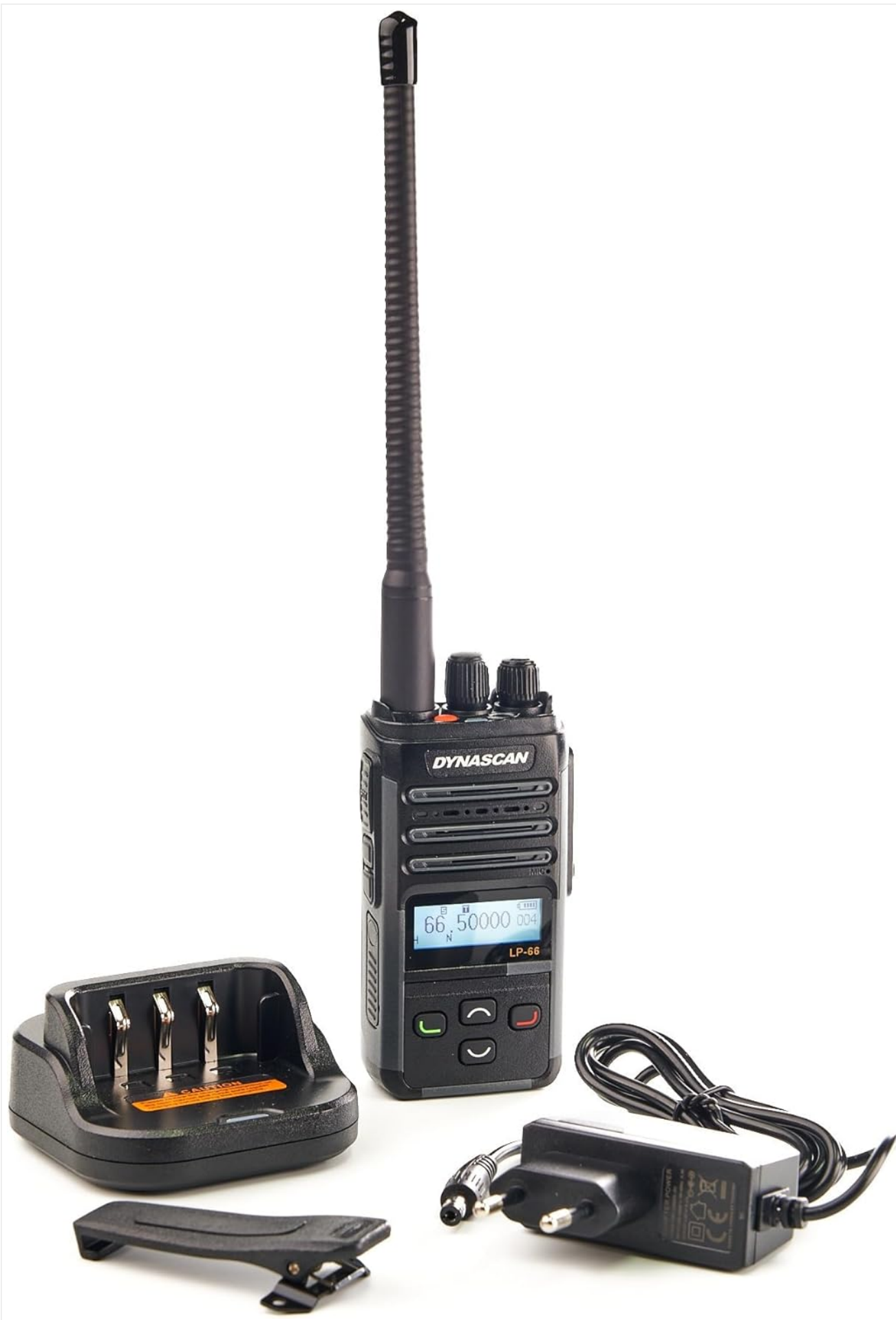
Figure 3.1: The Dynascan LP-66 walkie-talkie shown with its complete set of accessories, including the radio unit, battery, charger, power adapter, belt clip, and hand strap.
