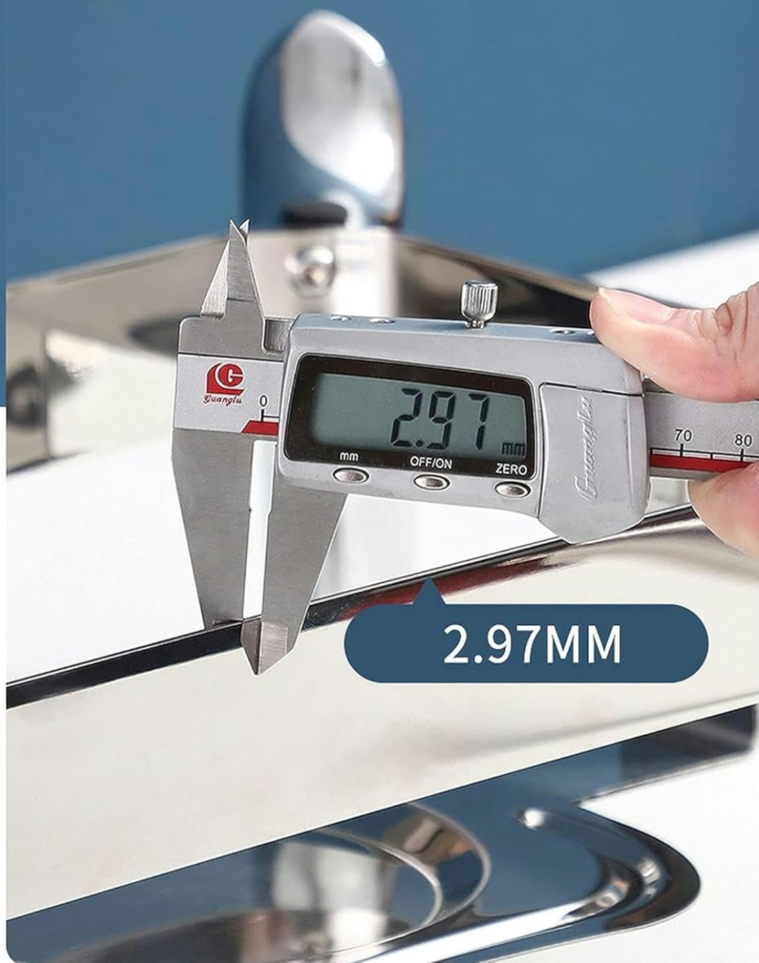
Figure 7: A close-up view demonstrating the thickness of the stainless steel material, measured at 2.97mm, highlighting the product's durable construction.
