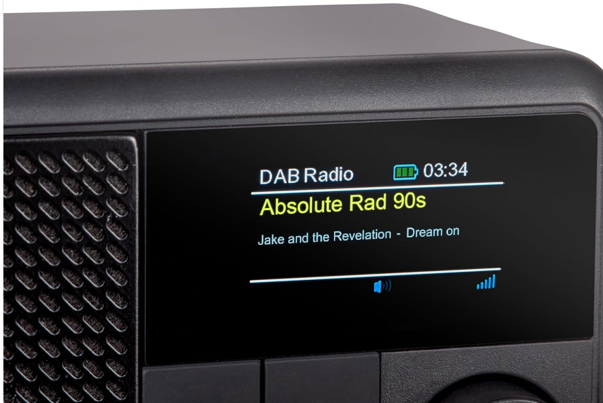
Figure 6.4: The 1.47-inch TFT color display showing radio information.
