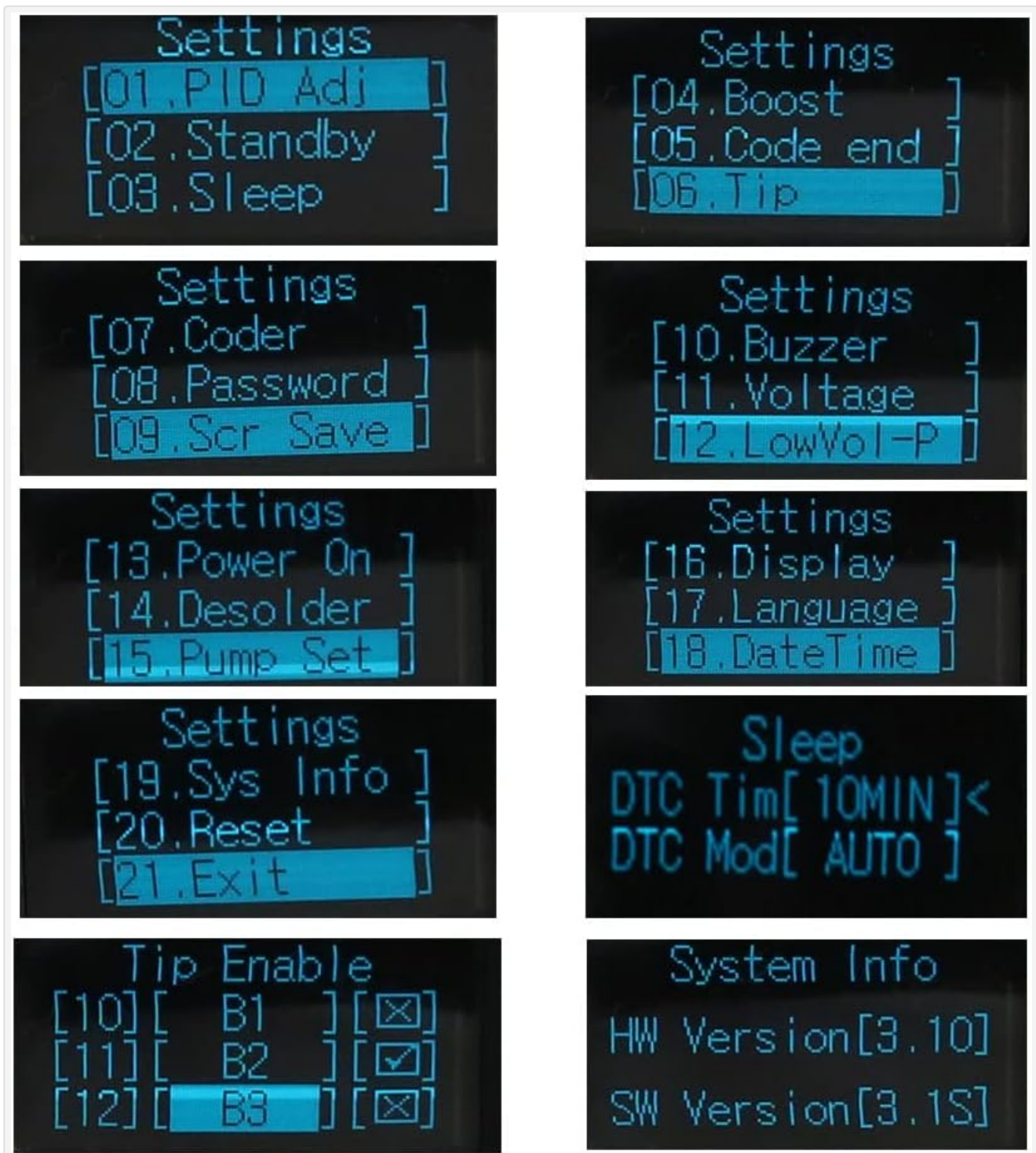
Figure 7.1: OLED Display Menu Options.
