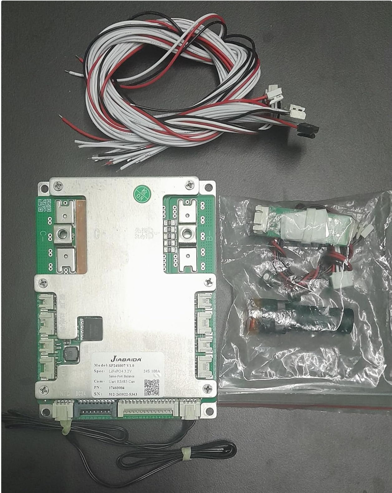
Figure 3.1: JBD Smart BMS unit with included balance wires, NTC sensors, and switch.
