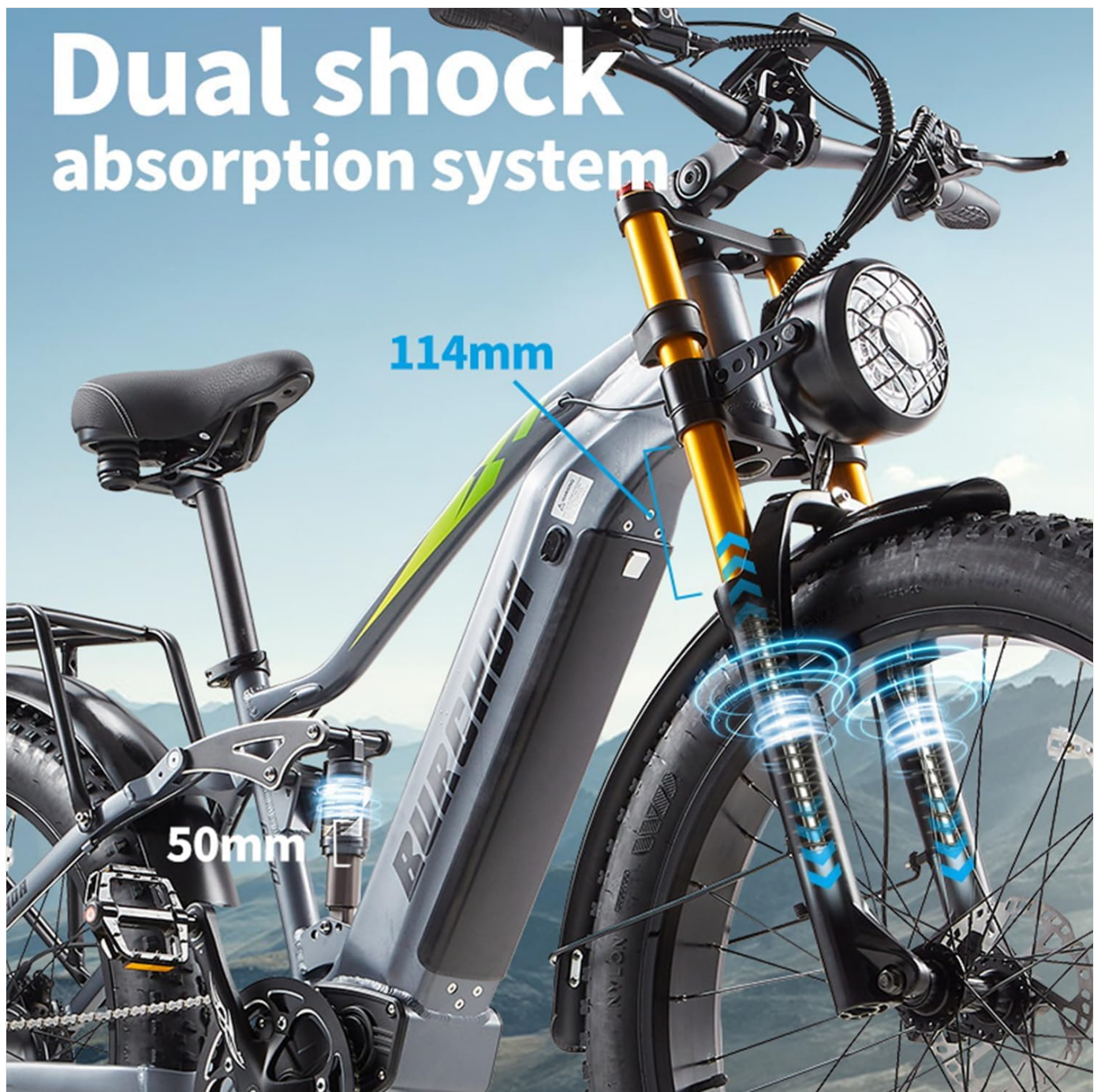
Figure 5.5: The dual shock absorption system, featuring a front fork with 114mm travel and a rear soft-tail suspension for enhanced comfort.
