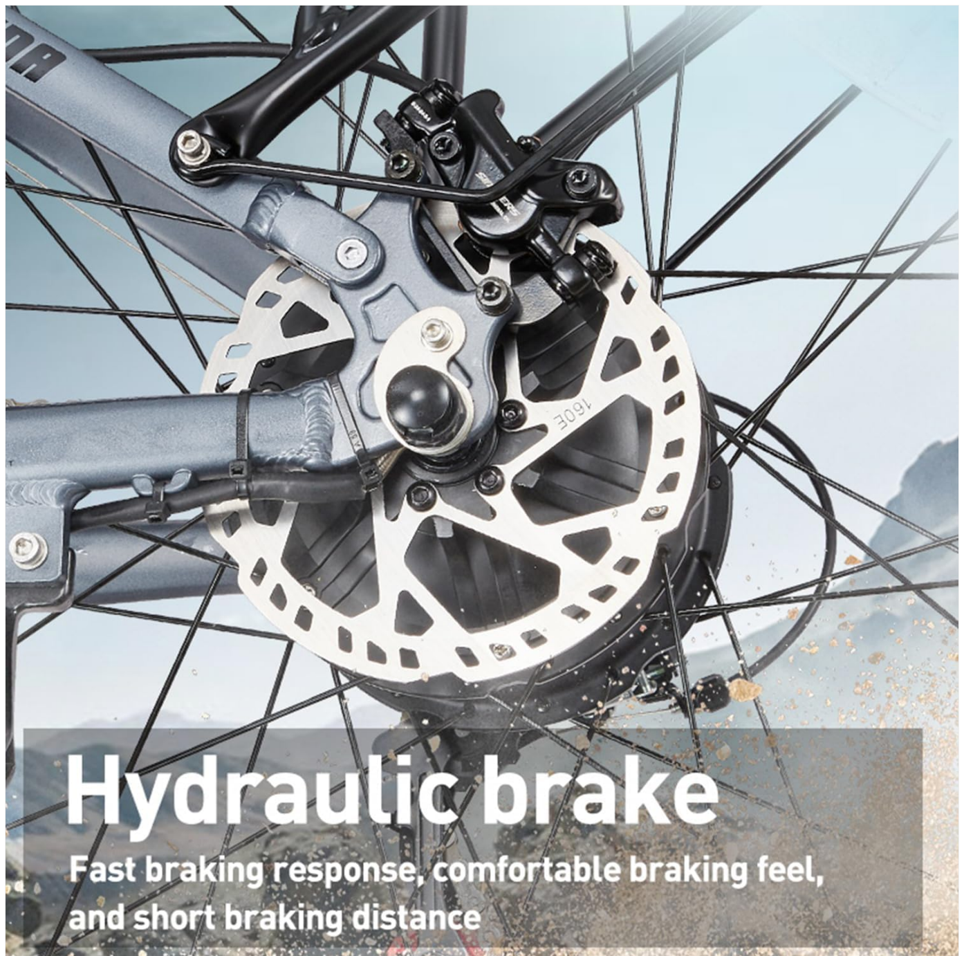
Figure 5.4: The hydraulic disc brake system, providing fast and stable braking with a motor power cut-off function.
