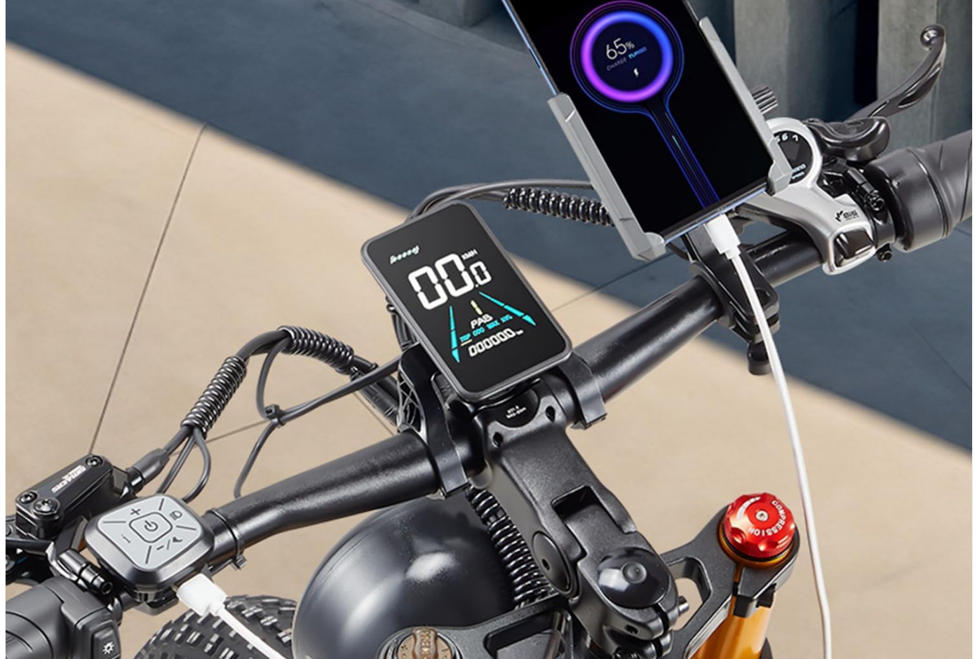
Figure 5.3: The Yolin Color LCD display, showing battery level, speed, and other ride data. It is IP65 waterproof.
