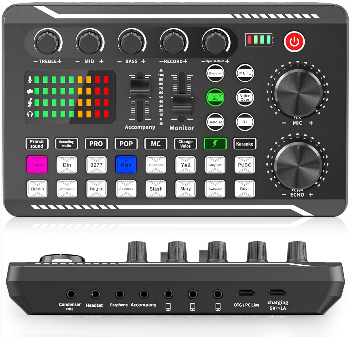
Detailed views of the F998 Live Sound Card, showing the control knobs and buttons on the front, and the various input/output ports on the rear for microphones, headphones, and devices.
