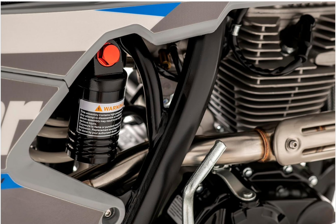
Figure 3.3: Detail of the rear suspension and chain drive system.
