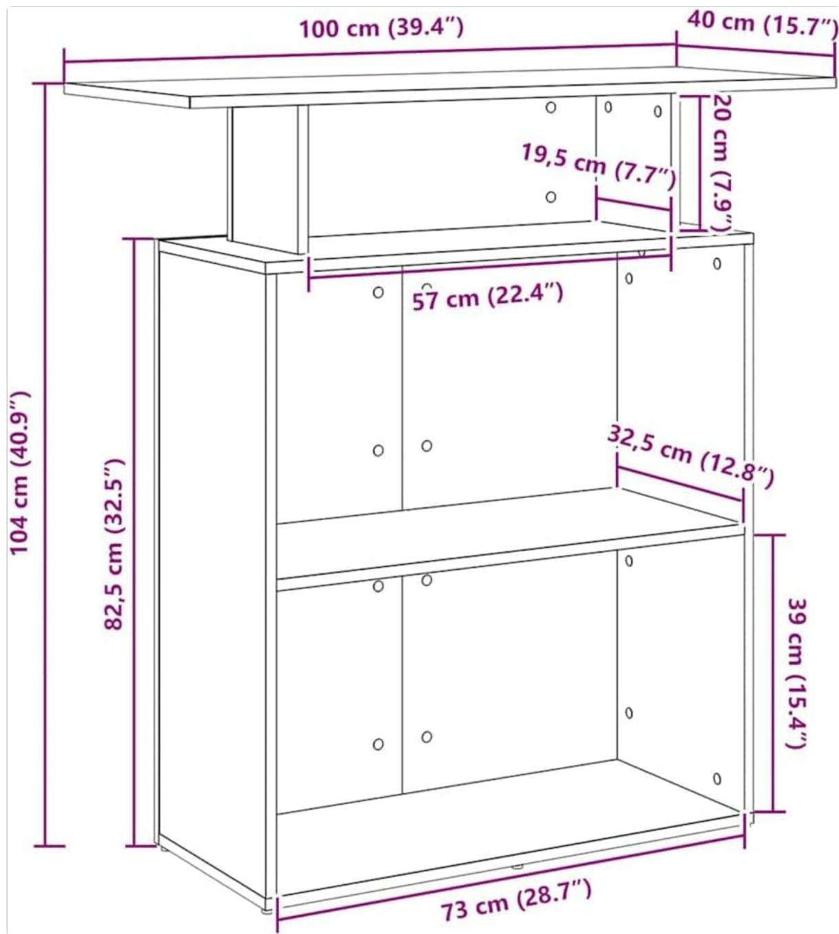
Image description: A technical drawing illustrating the full dimensions of the reception desk, including overall height (104 cm / 40.9"), length (100 cm / 39.4"), and width (40 cm / 15.7"), along with internal shelf and counter measurements.
