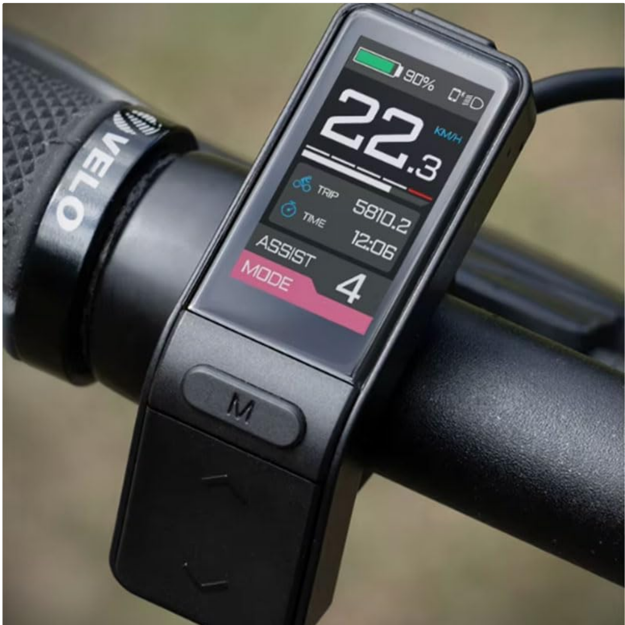
Image 7.1: The SW102/T display shown in a water environment, indicating its IPX5 waterproof rating.
