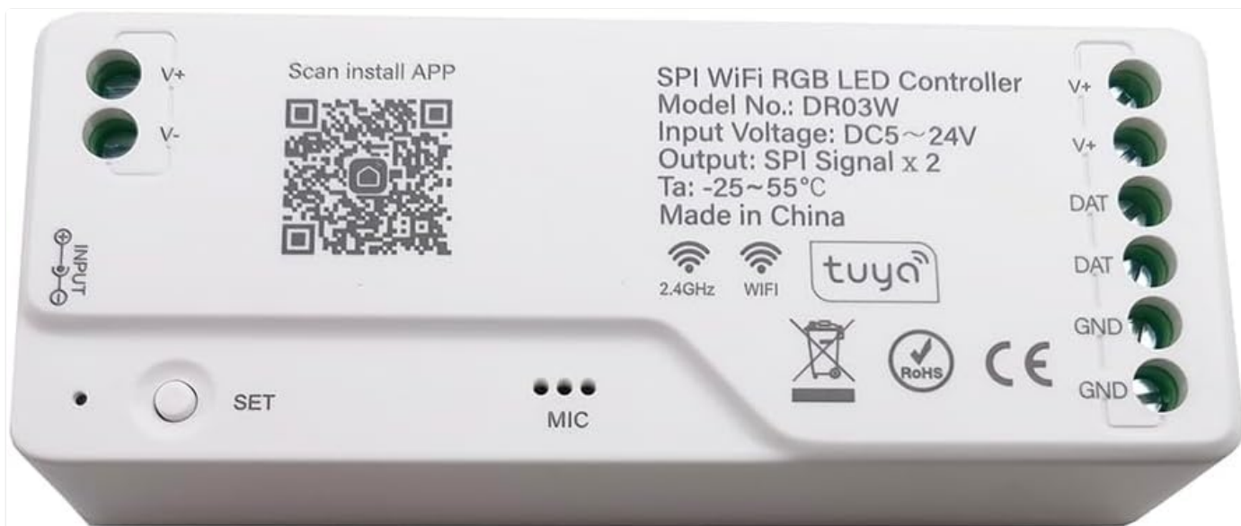
Image: Top view of the DR03W controller. Key features include the V+ and V- input terminals, a DC input jack, a 'SET' button for pairing, a 'MIC' (microphone) for music synchronization, and output terminals (V+, DAT, GND). A QR code for the Smart Life app is also visible. The link for the app is https://smartapp.tuya.com/smartlife .
