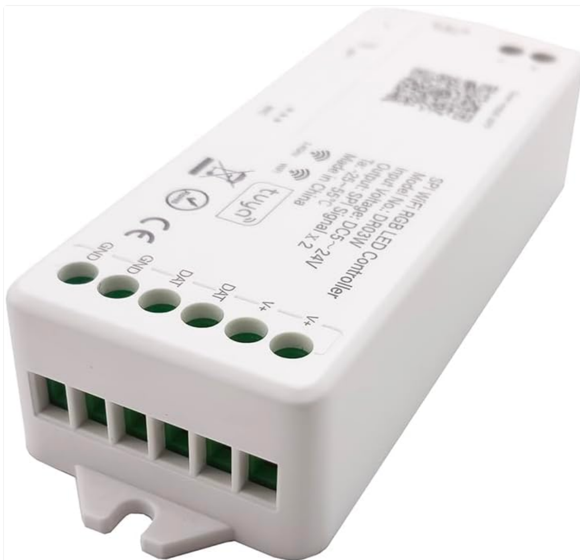
Image: An angled view of the DR03W controller, highlighting the screw terminals for both power input (V+, V-) and LED strip output (V+, DAT, GND).
