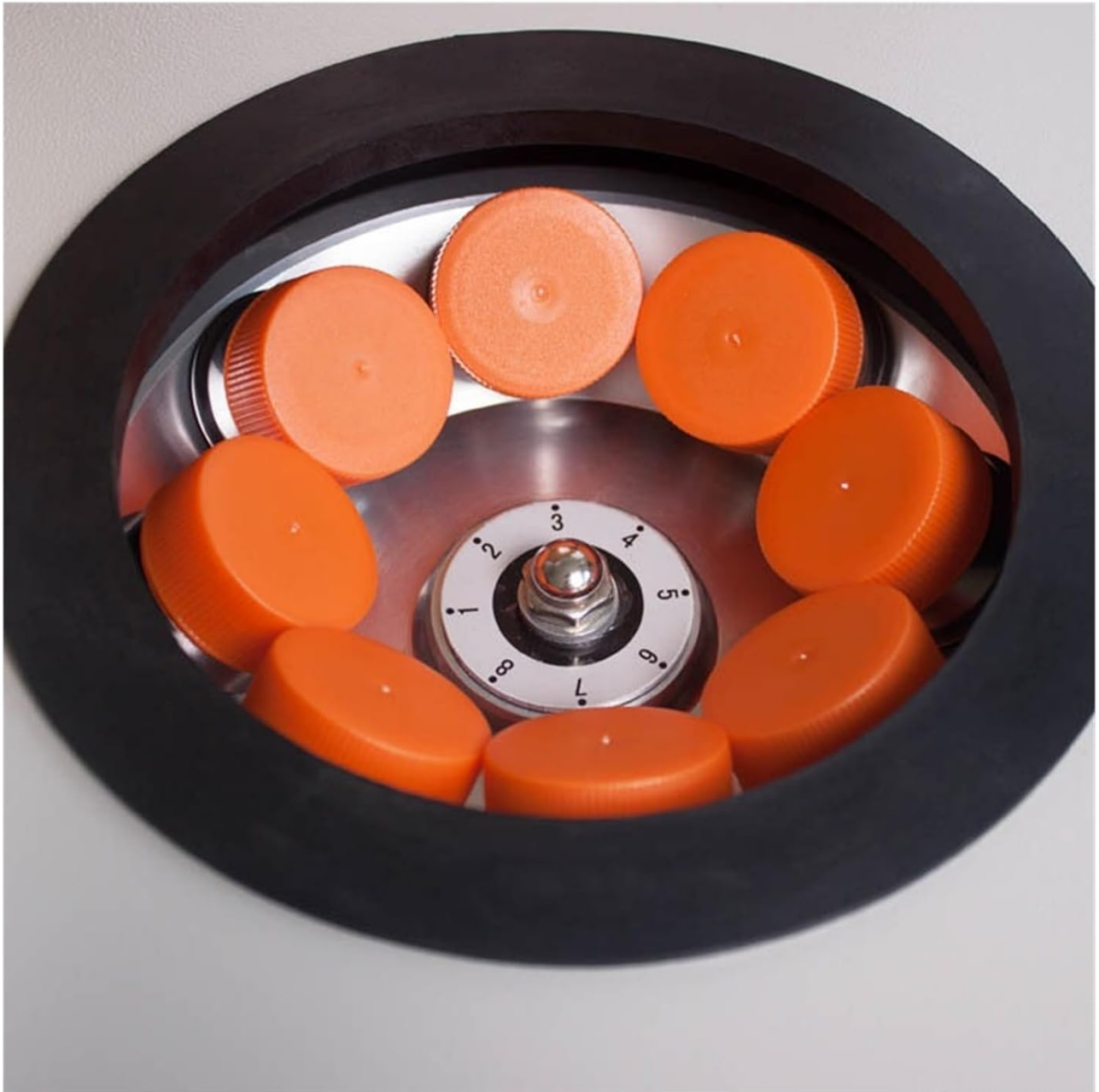
Figure 3.3: Rotor with Sample Tubes. A detailed view of the centrifuge rotor, showing six positions, each occupied by an orange-capped sample tube, ready for centrifugation.
