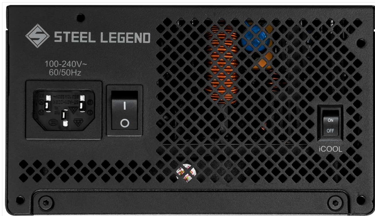
Image: Rear panel of the power supply, indicating the main power switch and iCool fan control switch.
