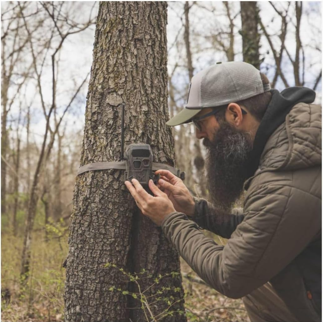
Figure 3.1: Proper camera mounting using the adjustable tree strap.
