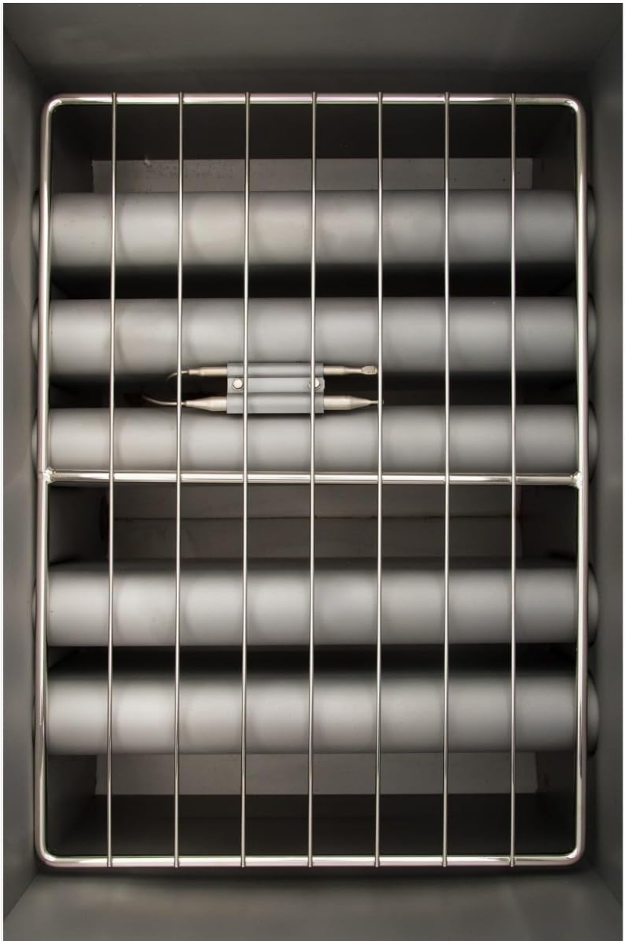
Image 5.1: Top-down view of the oil tank, showing the heating tubes and the rack that supports the frying baskets. Regular cleaning of this area is important.
