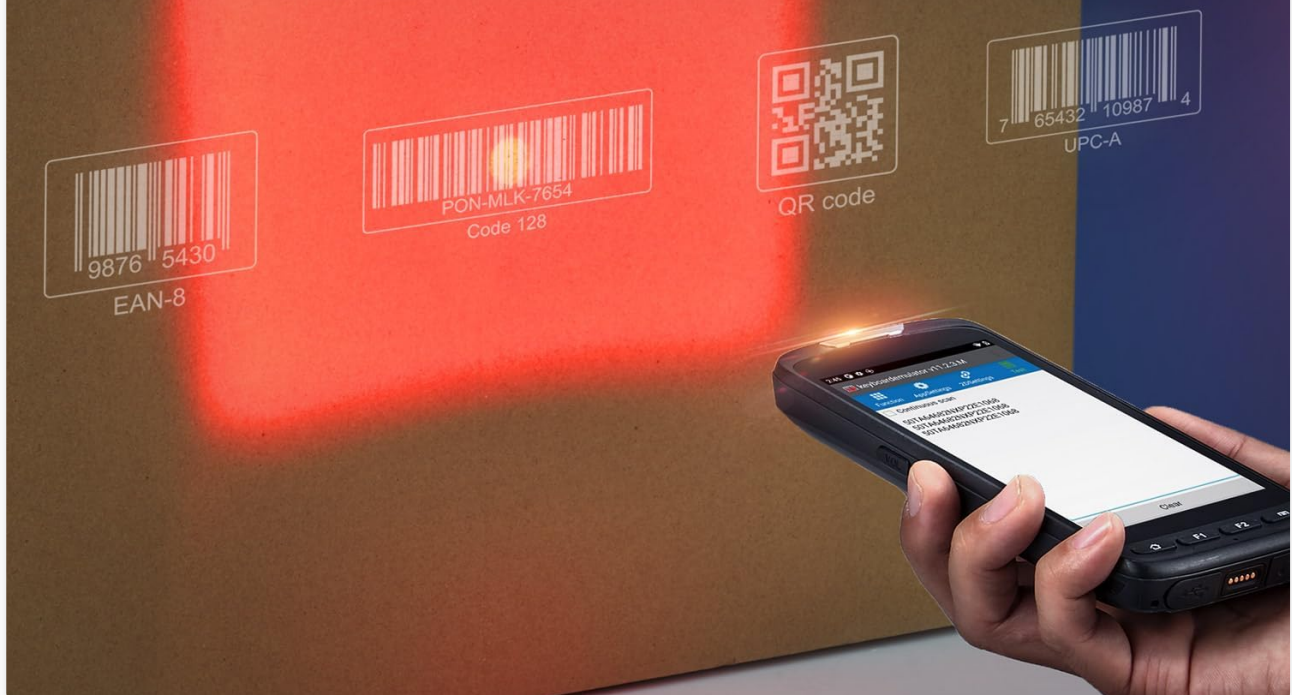
Figure 2.3: Image demonstrating the Zebra SE4710 scanner engine in action, accurately reading different types of barcodes and QR codes on a package.
