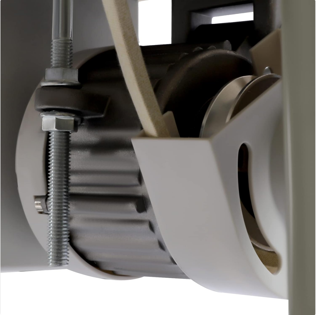
Image: A close-up view of the motor's pulley and the threaded rod with nuts used for adjusting belt tension.
