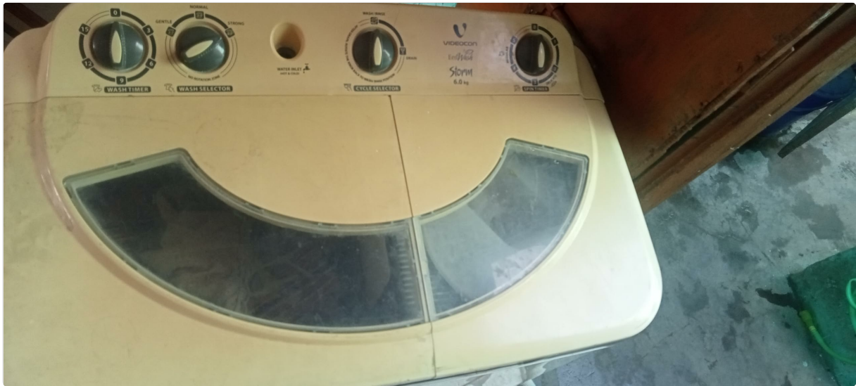
Figure 1: Front view of the Videocon Storm 6.5kg Semi-Automatic Top-Loading Washing Machine. This image displays the overall design, including the wash tub, spin tub, control panel, and water inlet.
