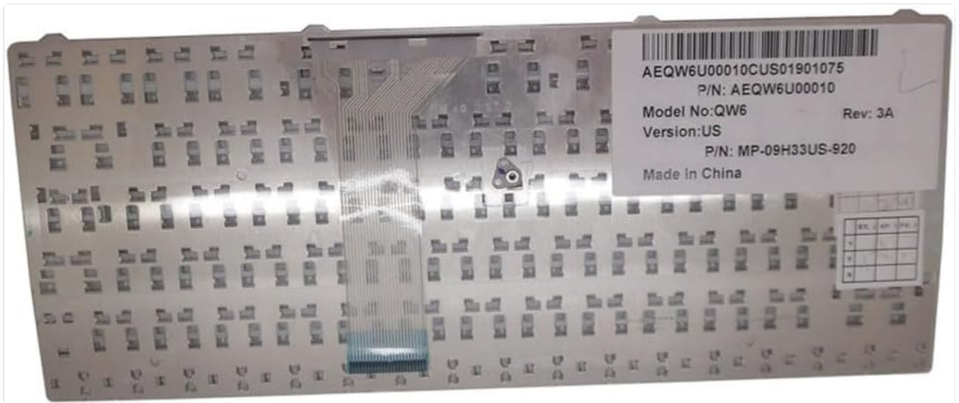
Image: Rear view of the replacement keyboard, highlighting the flexible ribbon cable connector and the various mounting points. This view is important for identifying the correct orientation and connection method during installation.
