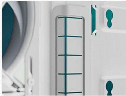
Figure 5: Locations for 2.5" SSDs and 3.5" HDDs.
