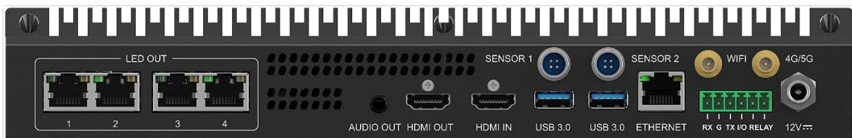
Image 3.2: Rear view of the EnhanBili MBOX600 Pro LED Screen Controller. This image shows the rear panel with LED OUT ports, Audio Out, HDMI Out, HDMI In, USB 3.0 ports, Ethernet port, Sensor ports, WiFi and 4G/5G antenna connectors, and the 12V power input.
