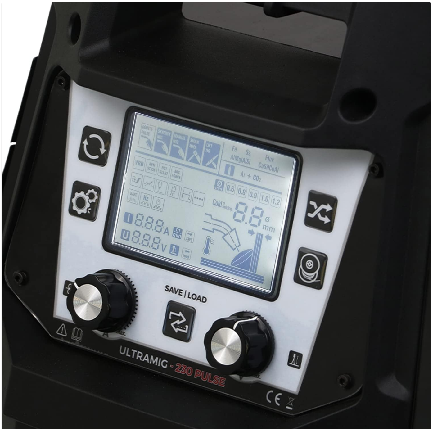
Figure 4.1: The ULTRAMIG 230 control panel, showing the main display and adjustment knobs.
