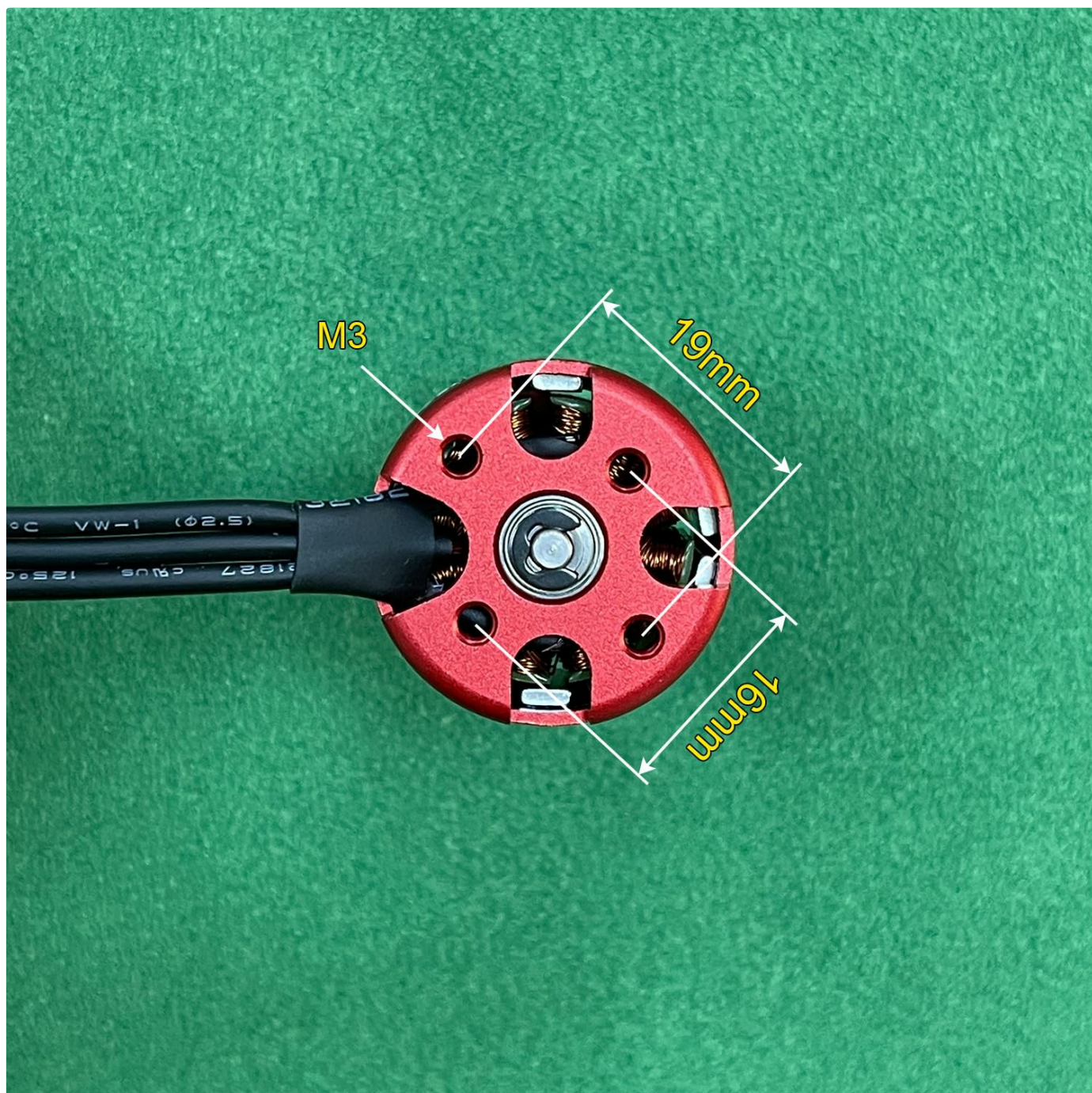
Image: Bottom view of the motor showing the 16mm and 19mm mounting hole patterns.
