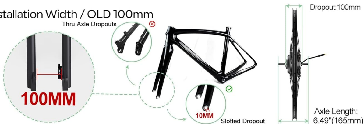
Image: Wheel size compatibility and front fork installation dimensions.
