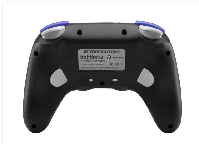
Image: Rear view of the BattlerGC Pro controller, highlighting the BT/2.4G mode switch and P1/P2 back buttons.
