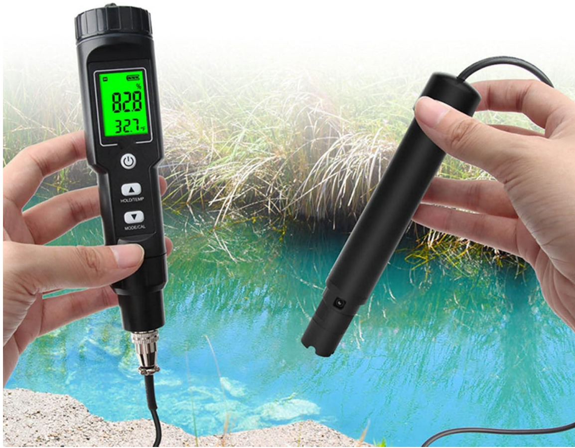
Figure 3.3: A close-up view of the ANKROYU DO9100's digital display and control buttons, including Power, HOLD/TEMP, and MODE/CAL.
