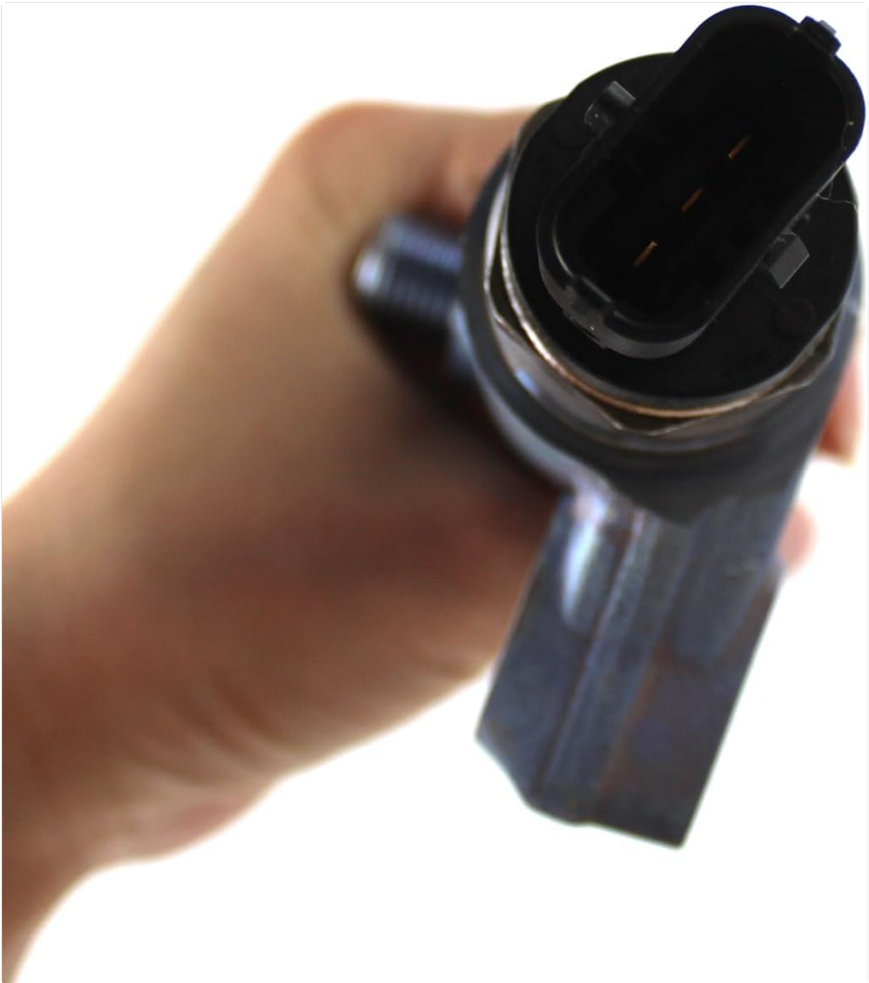
Figure 4: Close-up view of the electrical connector on the Common Rail Assembly.
