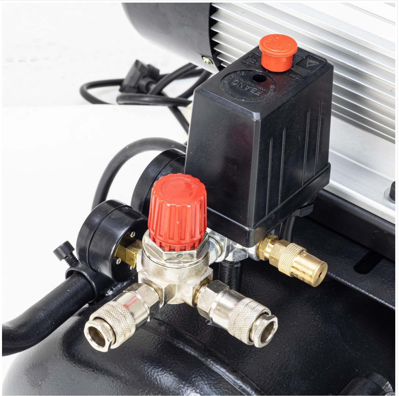
Figure 3.4: Close-up view of the quick-connect air outlets and the pressure switch, which controls the compressor's automatic on/off cycle.
