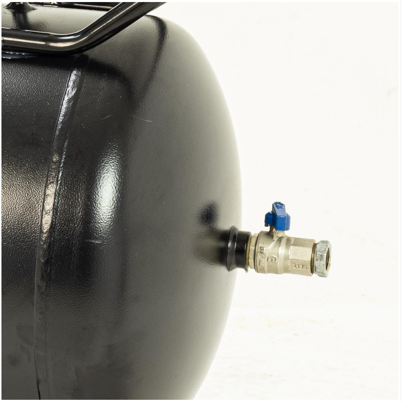
Figure 3.5: Close-up view of the tank drain valve located at the bottom of the air receiver, essential for draining condensed moisture.
