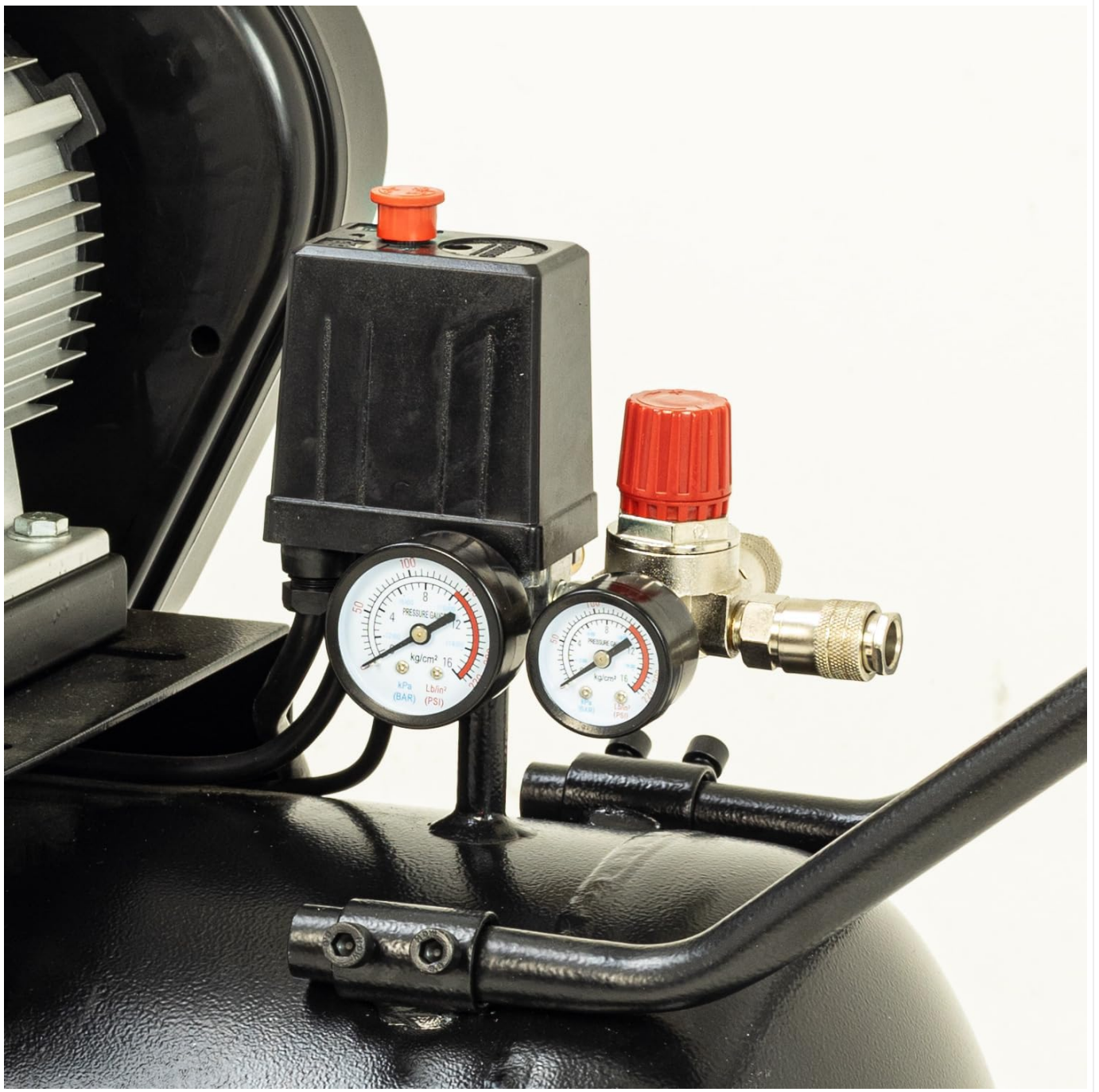
Figure 3.3: Close-up view of the pressure gauges and air pressure regulator, used for monitoring and adjusting output pressure.
