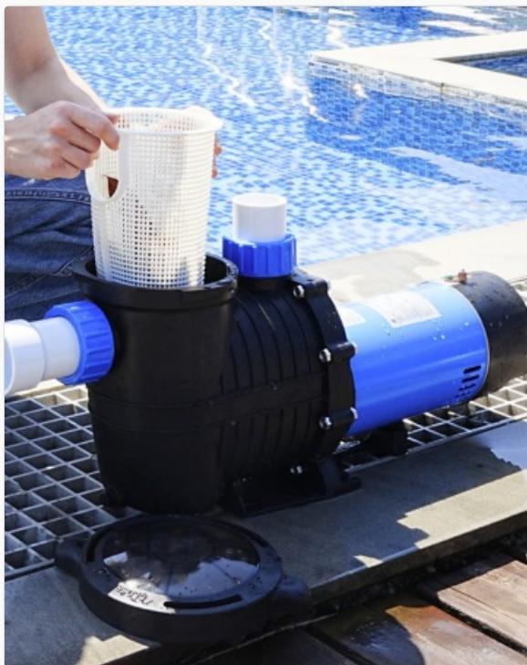
Image: Demonstrating the process of filling the filter basket with water to prime the pump.
