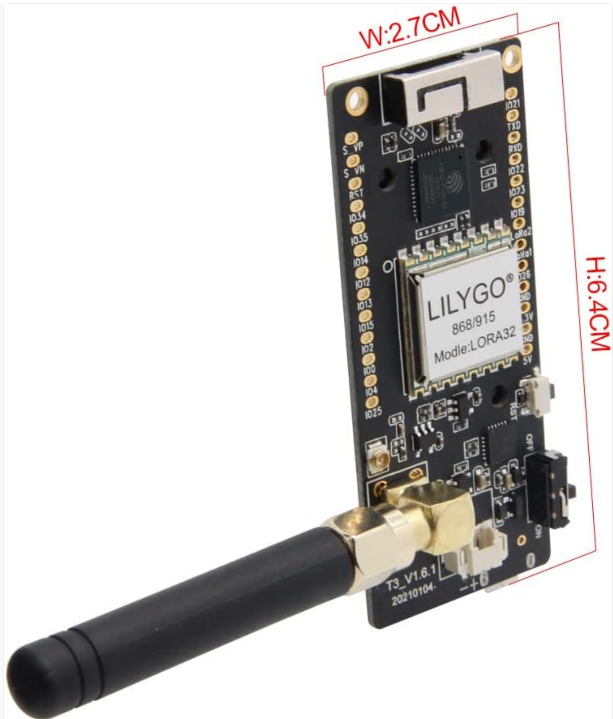
Figure 4.1: This image displays the LILYGO ESP32 LoRa32 V2.1_1.6.1 wireless module with its antenna connected, showing its approximate dimensions: width 2.7cm and height 6.4cm. The module features an integrated OLED display and various pin headers.
