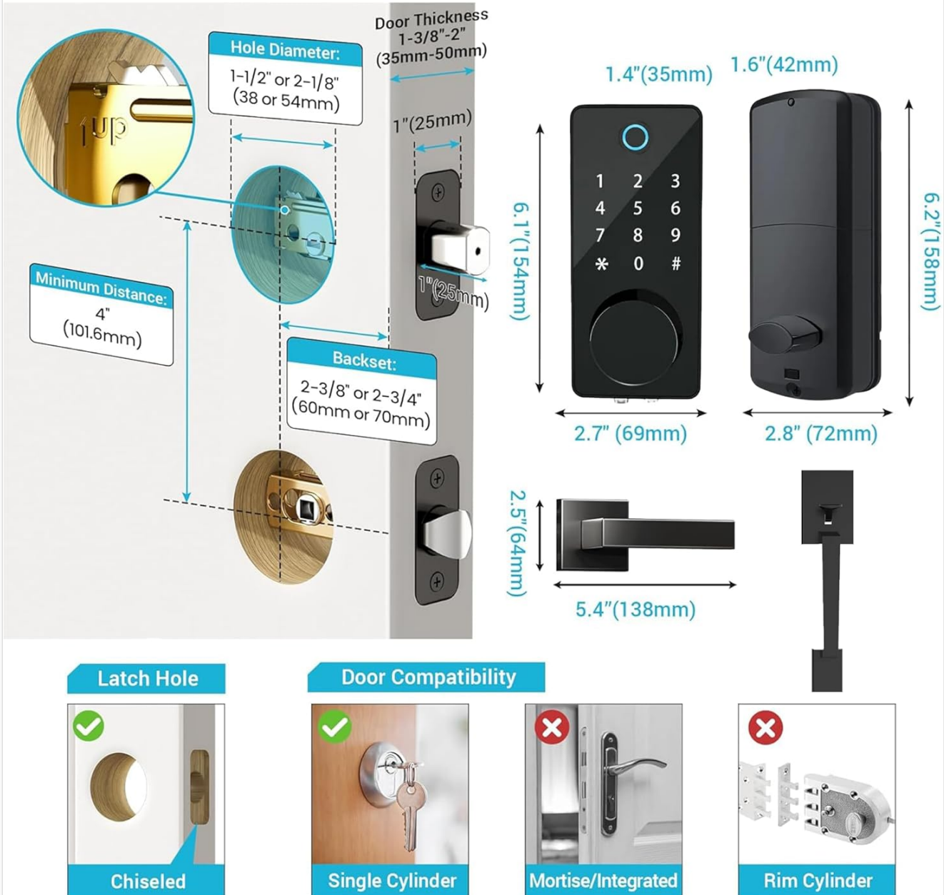
Image 3.1: Diagram illustrating required door dimensions (thickness, hole diameter, backset, minimum distance) and compatible door types (single cylinder) for installation.
