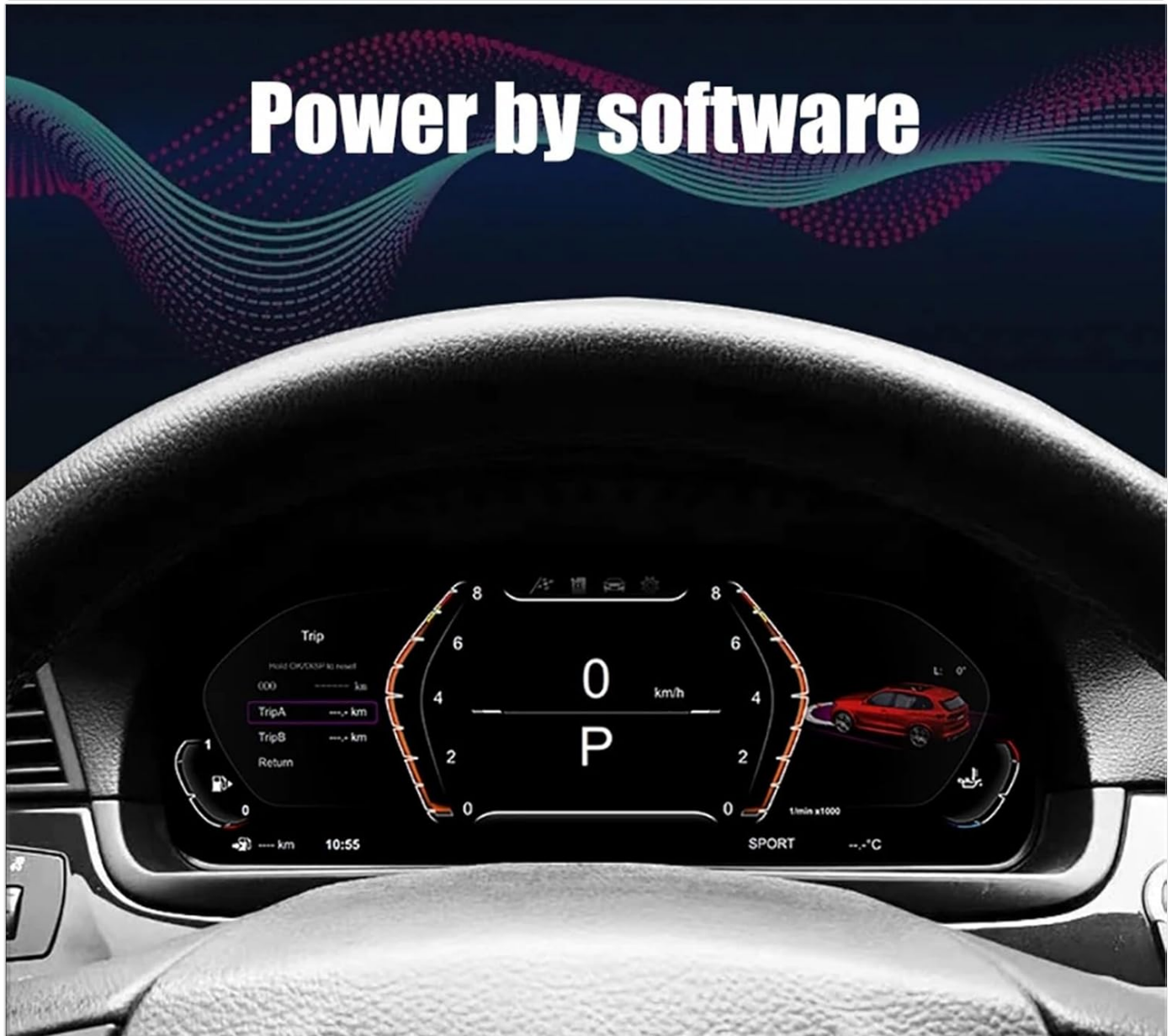
Figure 2.1: The 12.3-inch LCD Digital Virtual Cockpit Cluster installed in a vehicle dashboard, demonstrating its integration and display alongside the original infotainment screen.
