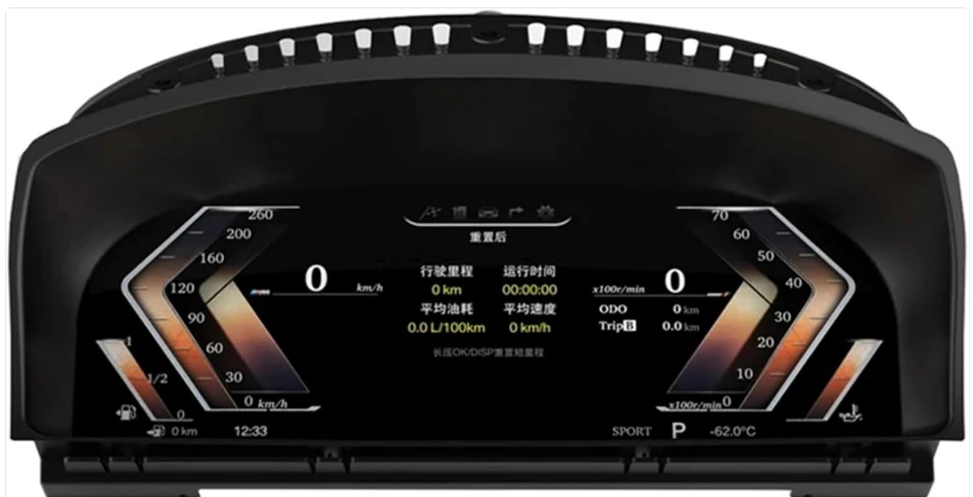
Figure 3.2: Efficiency display mode with detailed trip and fuel economy data.
