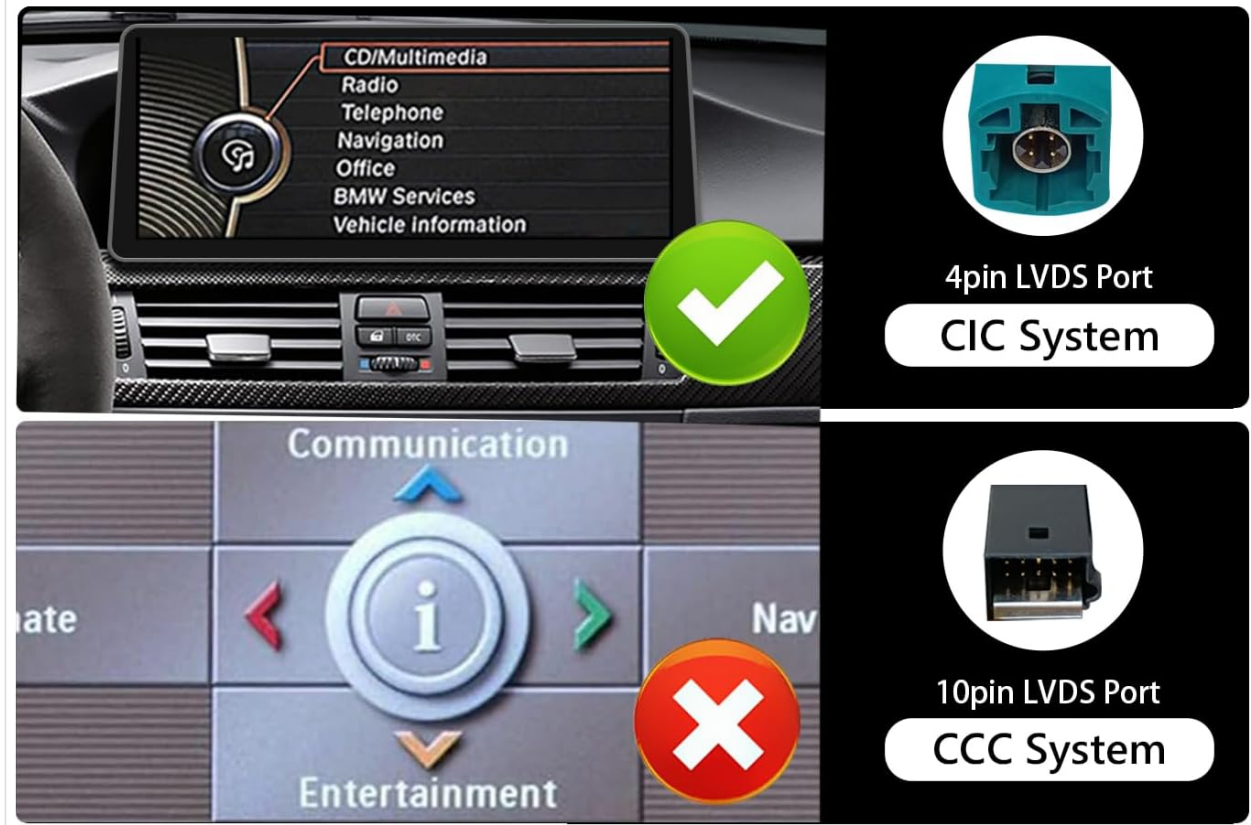
Figure 3.1: Identifying CIC vs. CCC Systems. Ensure your vehicle has a CIC system (4-pin LVDS port) for compatibility.
