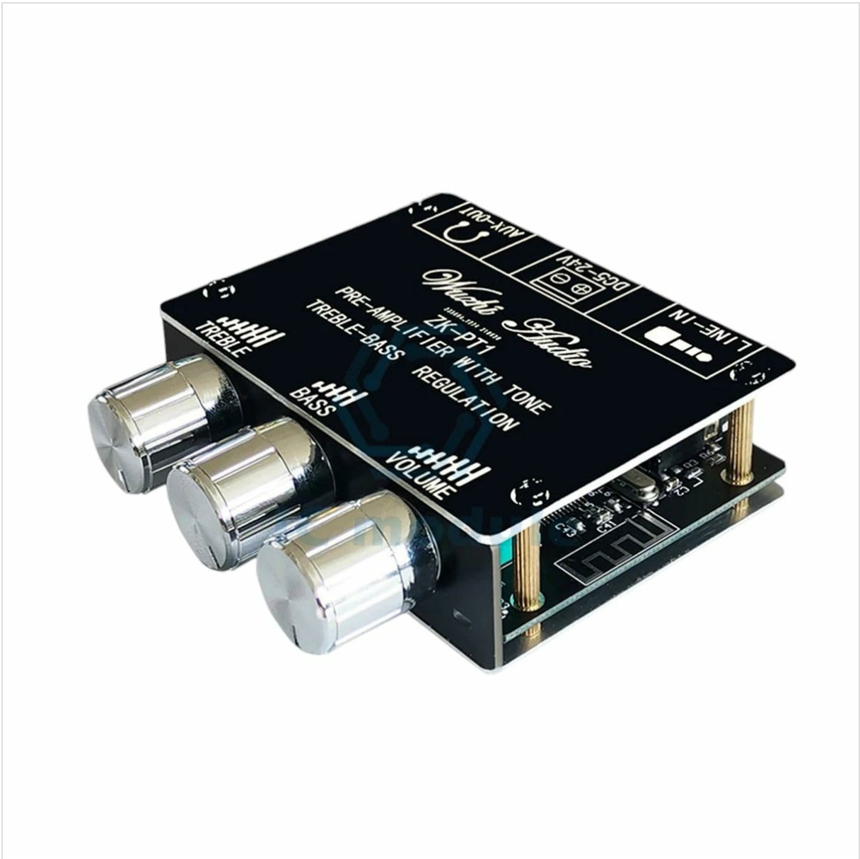
Figure 1: FICEMETOI ZK-PT1 Audio Receiver Decoder Board. This image displays the top view of the ZK-PT1 board, highlighting the three control knobs for Treble, Bass, and Volume on the left side. On the right side, the input/output ports are visible, including DC 5-24V power input, LINE-IN audio input, and AUX-OUT audio output. The board is black with white text labels.
