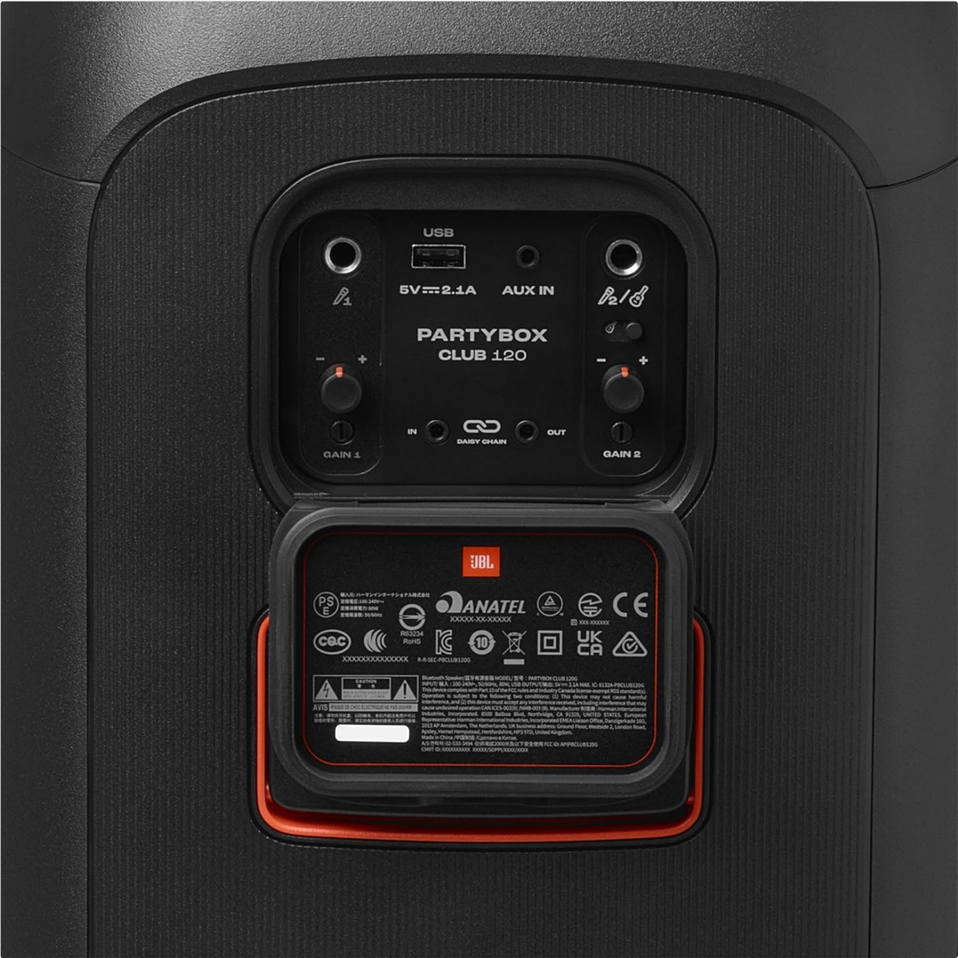
Figure 4: Rear panel with USB, AUX In, Microphone/Guitar inputs, and Daisy Chain In/Out ports.
