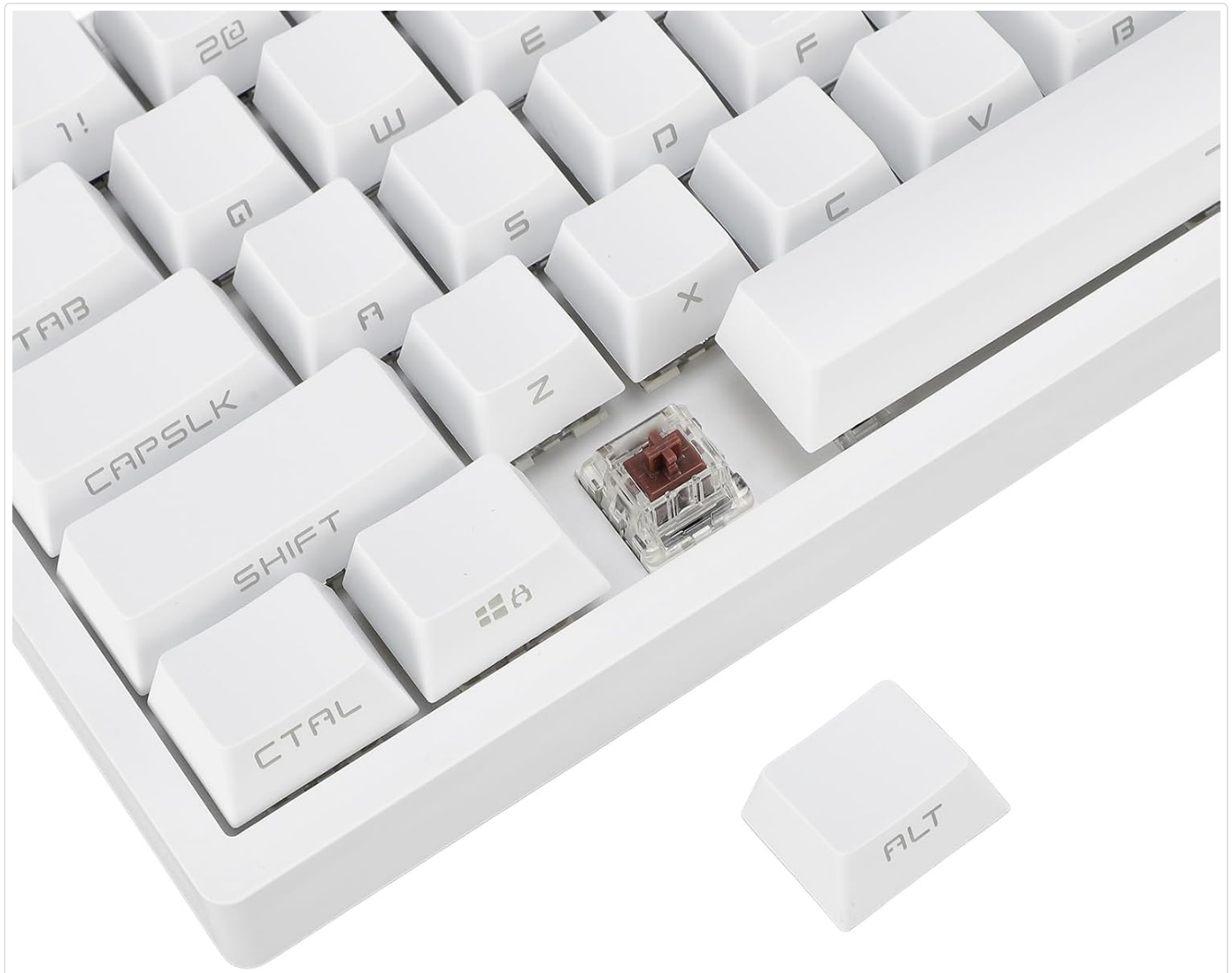
Image 5.1: A brown mechanical switch exposed after removing the keycap, demonstrating the hot-swappable feature.
